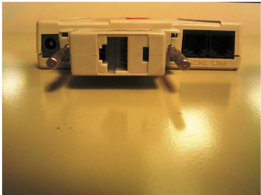
Figure 7.5. Modem Connections. Left to right: Power, Serial RJ-45, Phone Set, POTS Line.
