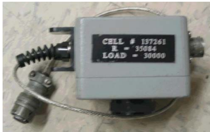
Figure 10.7 Shunt Resistor Box
