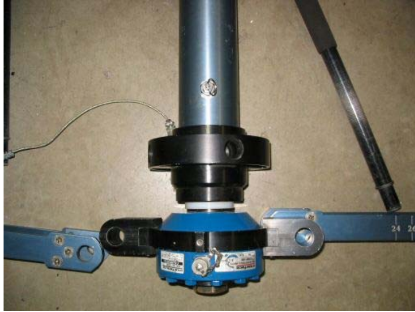
Figure 10.18 Attachment of Small I-beams to Load Cell
