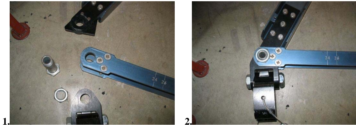
Figure 10.16 Assembly of Small I beam Connection
