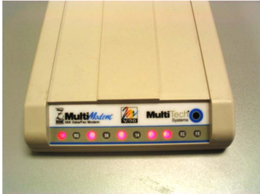
Figure 7.4. Modem actively transmitting. Carrier Detect (CD), 56, OH, and CR lit. Transmit Detect (TD), Receive Detect (RD), and Error Correction (EC) blinking.
