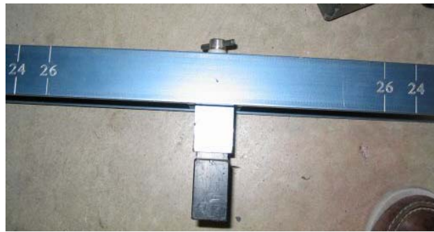
Figure 10.17 Insertion of Rail Height Adjustment Blocks
