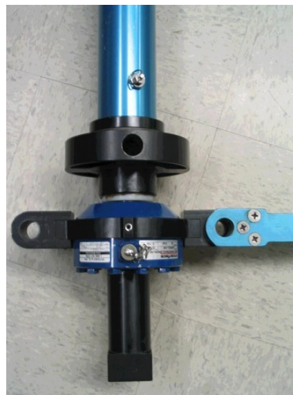
Figure 10.26 Attached Load Cell Lateral Adaptor
