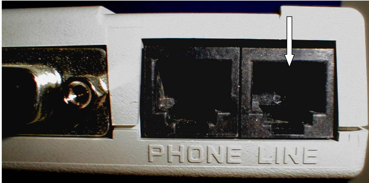
Figure 7.9. Plug the phone jack into the “LINE” socket.
