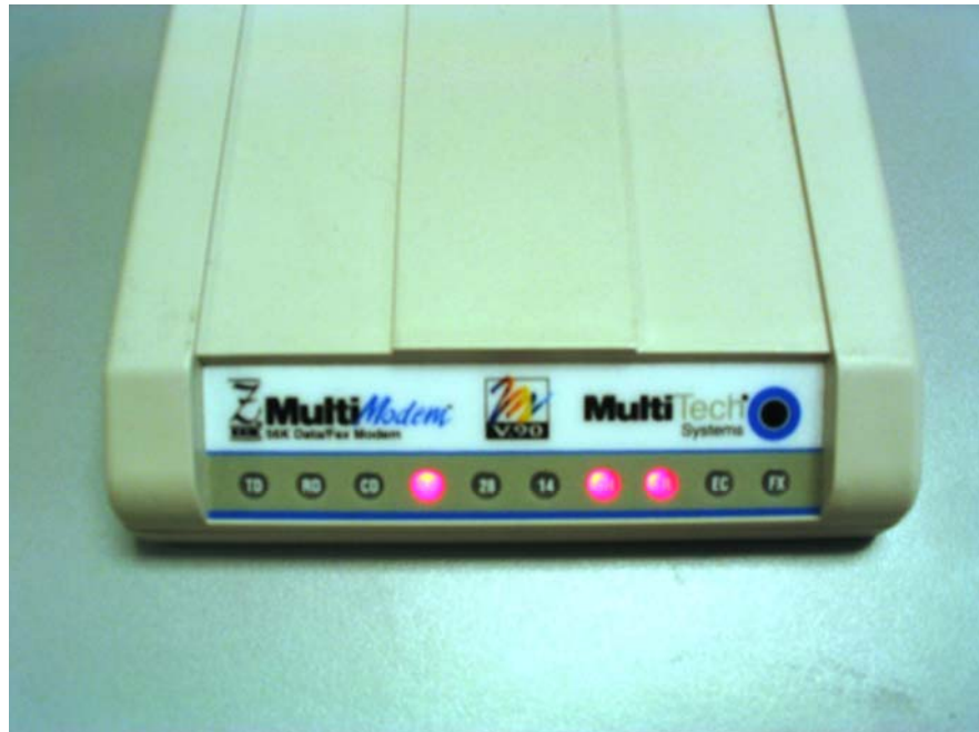
Figure 7.3. Modem off-hook without data passing. 56, TR, and Off-Hook (OH) lit.
