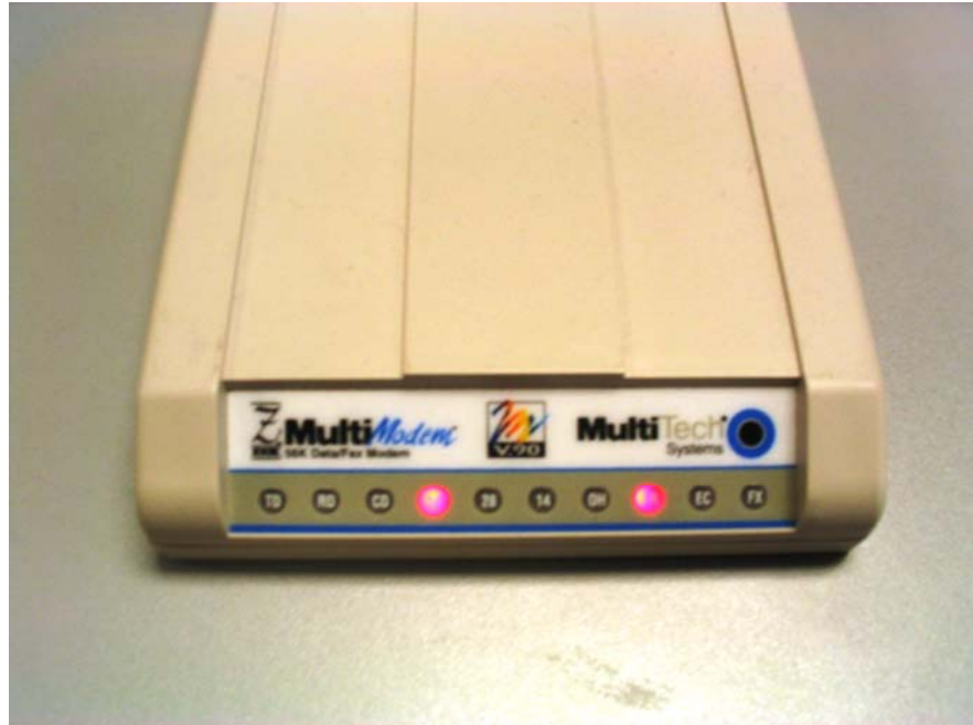
Figure 7.2. Modem idle with Transmit Ready (TR) and 56K (56) lit.
