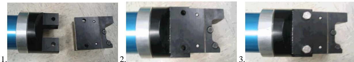
Figure 10.24 Attachment of U-shaped Lateral Adaptor
