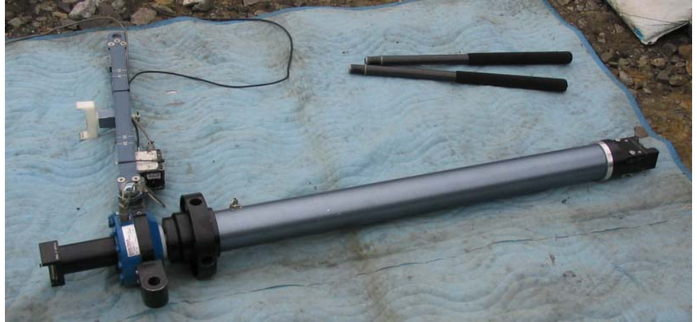
Figure 10.33. CalJack assembled for lateral calibration
