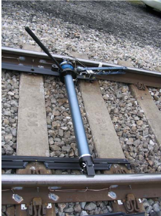
Figure 10.34. Lateral CalJack in proper position.
