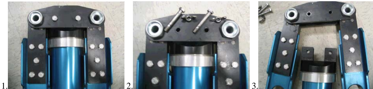
Figure 10.23 Removal of Large I-beams
