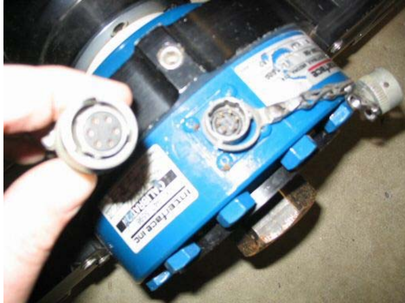
Figure 10.20 Connection of Shunt Resistor Box to Load Cell
