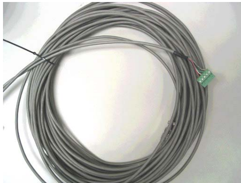
Figure 10.11 Interface Connection Cord
