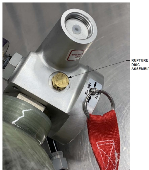
Figure1: Example of the location of Rupture Disc on reservoir
