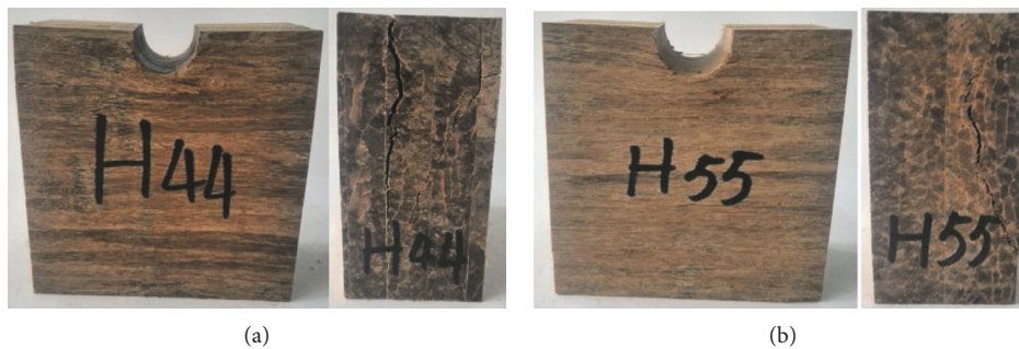
FIGURE 4: Typical failure mode of the specimen.
