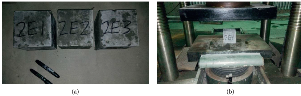
FIGURE 1: Compressive strength test. (a) Test specimen and (b) servo-controlled hydraulic testing machine.
