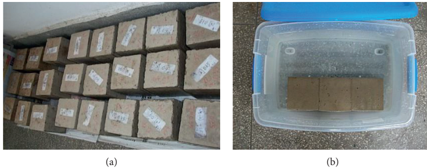
FIGURE 2: Test layout for sulfuric acid corrosion on concrete: (a) specimens and (b) soaking pool.
