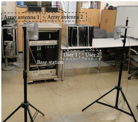
FIGURE 9: Implemented MU-MIMO test-bed.
