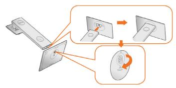
5 Lift the cover, as shown, to expose the VESA area for stand assembly.
