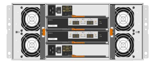
**Attention:** Possible equipment damage — If you replace a fan canister with the power turned on, you must complete the replacement procedure within 30 minutes to prevent the possibility of overheating the equipment.
