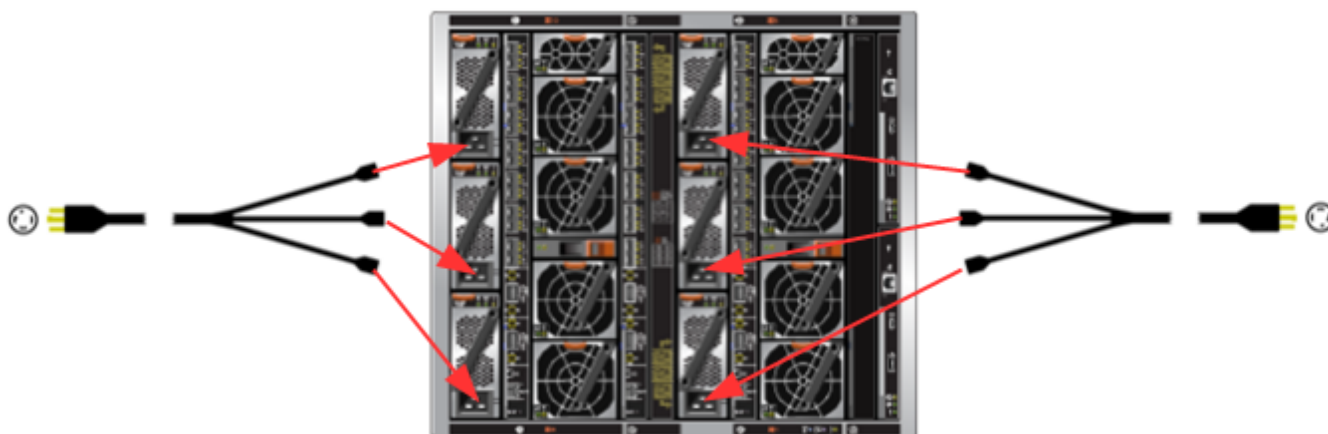
Figure 68: Line cord 00D7192 for use with Flex System with 6x PSUs installed
