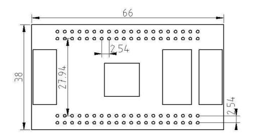
Figure 3: Dimensions of Sphinx-C100
