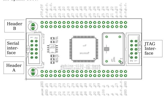
Figure 2: Sphinx-C100 connection diagram
