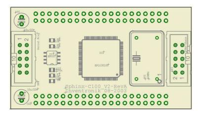
Figure 1: Top View of the Module Sphinx-C100
