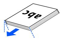
7. Place the originals into the ADF input tray facing up and with the top edge facing into the ADF. Insert the paper into the ADF until it meets resistance.
