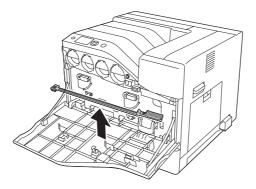
3. Insert the cleaning rod all the way into the hole under the photoconductor unit with its sponge facing down, and then slide it out.
