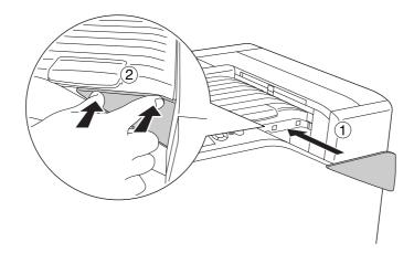
16. Remove the cover on the printer.
