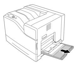
3. Load a stack of the desired paper with the printable surface facing down. Then slide the paper guides to get a snug fit.
