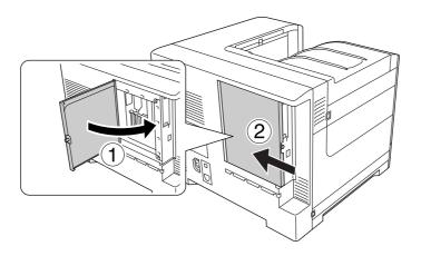
8. Fasten the back cover with the screw.
