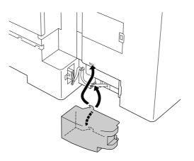
19. Attach the cable clamp of the cover L unit and plug the connector into the connector on the printer.
