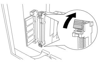
5. Confirm that the notch on the expansion memory module matches with that of the slot, and then firmly insert the top edge of the memory module into the slot until it stops.
