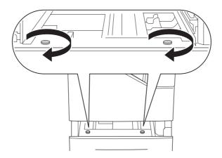
8. Attach the plate and fix the printer to the optional cassette unit with a screw.
