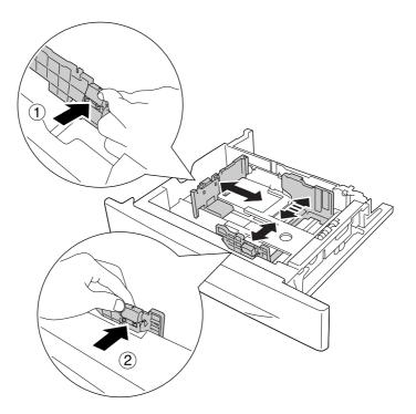
2. Pinch the knobs and slide the paper guides to accommodate the paper you are loading.
