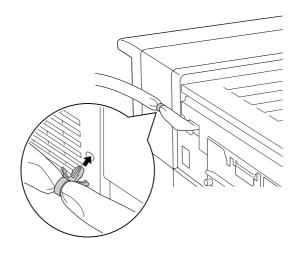
10. Install the stapler/stacker unit. Make sure that the cable is not stuck between the printer and the unit.
