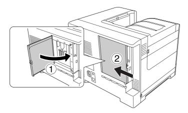
6. Fasten the back cover with the screw.
