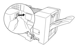
17. Attach the cable clamps of the stapler/stacker unit and plug the connector into the connector on the printer.
