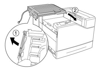
7. Insert the bracket as shown below and hold it in place.
