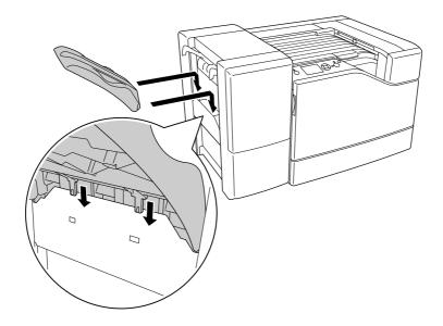
13. Install the stacker tray. Make sure that the two claws go as shown below.
