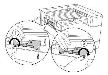
9. Attach the cable clamp.
