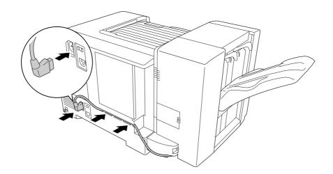
24. Reconnect the interface cable and power cord and turn the printer on.
