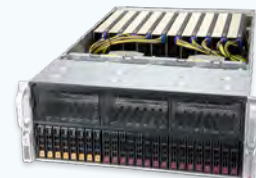
SYS-420GP-TNR Dual Root Configuration, PCI-E GPU
