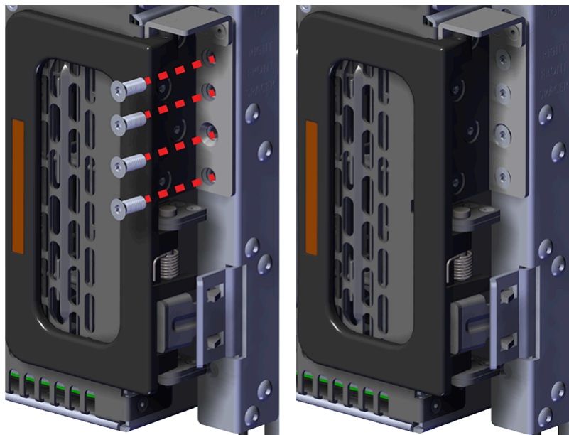
Figure 286: Shipping Bracket Screw Locations (CMA Lite)
