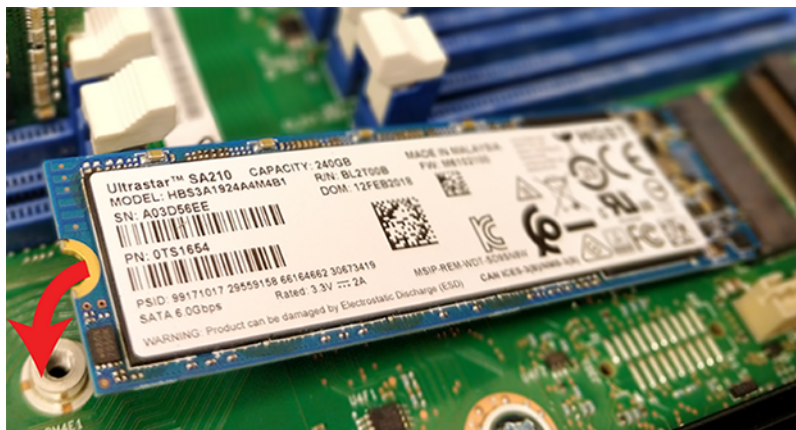
Figure 214: M.2 Install (Top)
