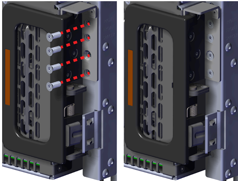
Figure 404: Shipping Bracket Screw Locations (CMA Lite)
