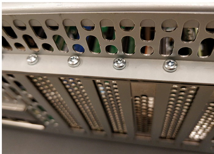
Figure 244: Add-In Card Screws
