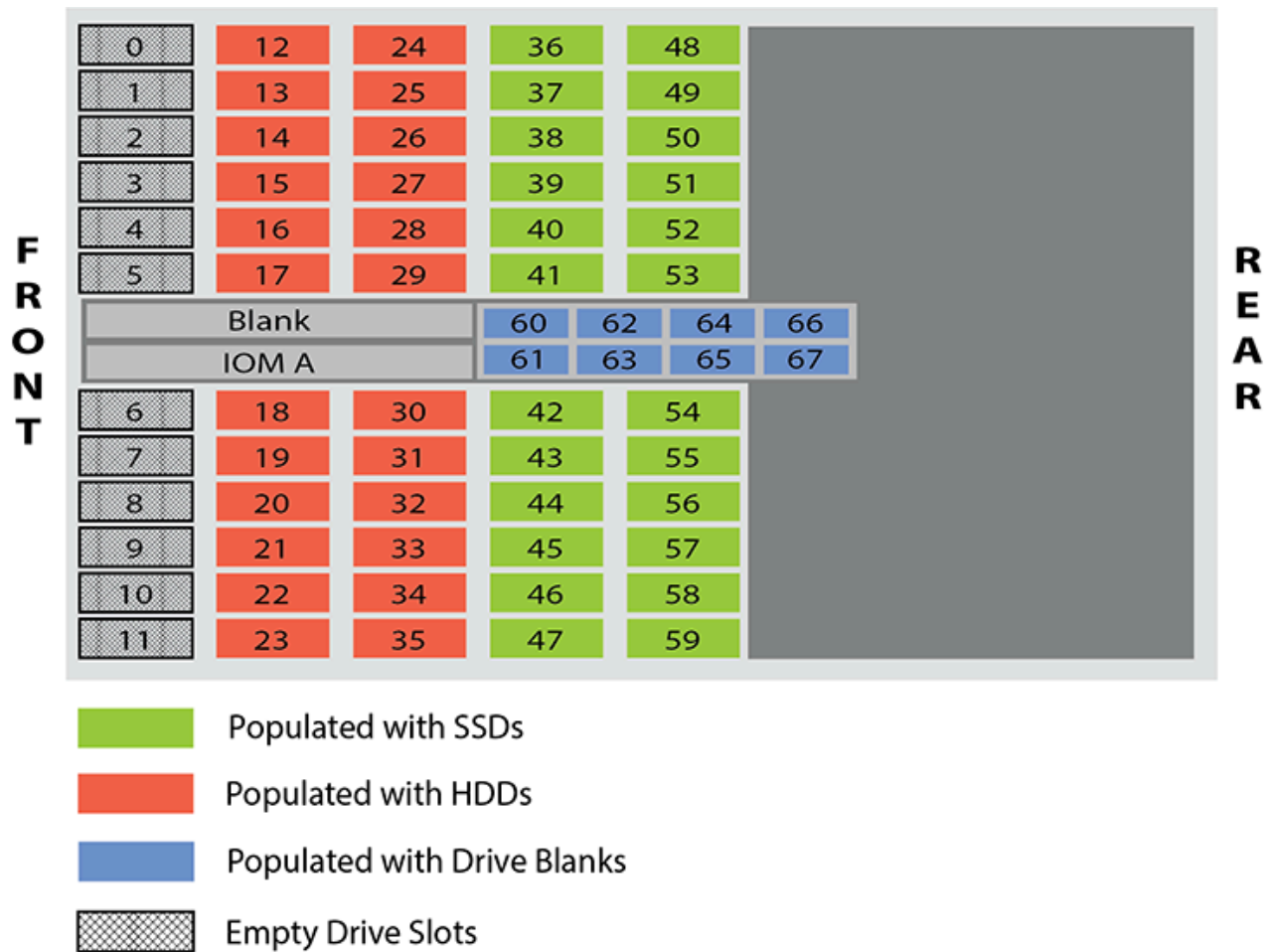
Figure 507: Minimum HDD and Maximum SSD Partial Population
