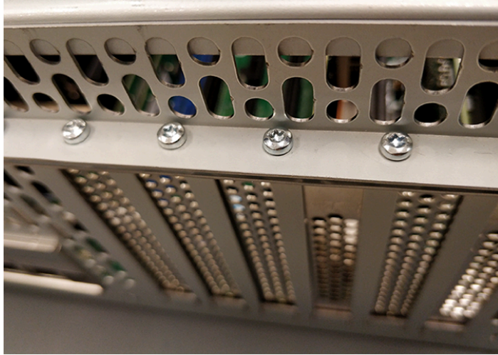
Figure 237: Add-In Card Screws
