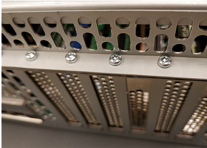
Figure 359: Add-In Card Screws
