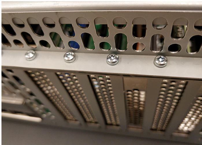
Figure 379: Add-In Card Screws
