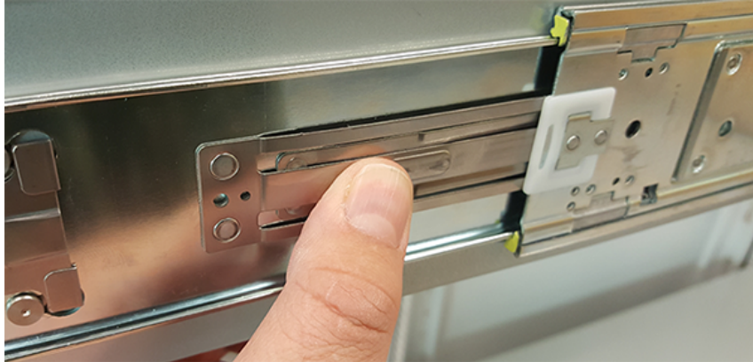
Figure 107: Inner Rail Safety Latch Release
