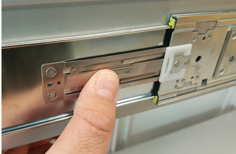
Figure 167: Safety Latch Release
