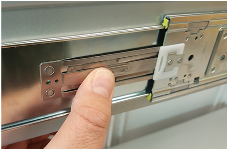
Figure 78: Safety Latch Release
