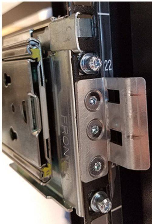
Figure 114: Rack Latch Bracket Installed
