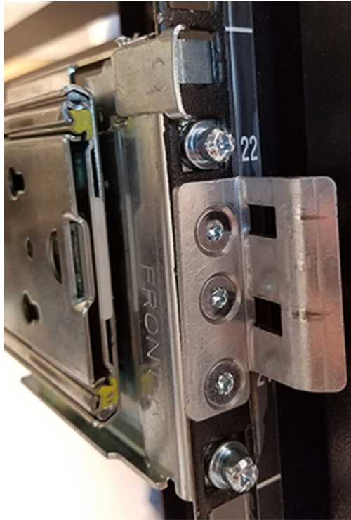
Figure 127: Rack Latch Bracket Installed
