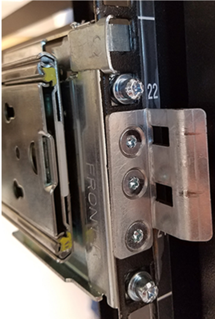
Figure 29: Rack Latch Bracket Installed
