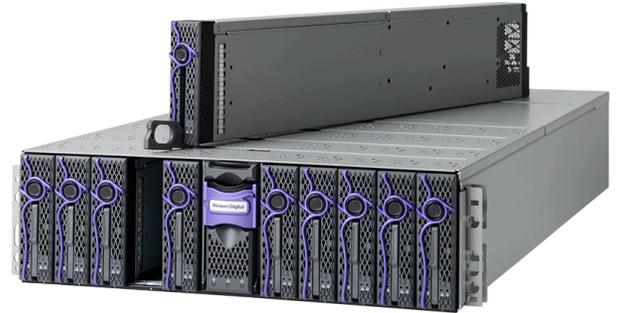
The maximum data storage capacity is 614TB<sup>1</sup> when leveraging a full set of 10 F3x00 fabric devices. The enclosure runs on an input voltage of 200V - 240V and consumes ~1400W of power under typical conditions. It requires a maximum of 1600W at full load.
