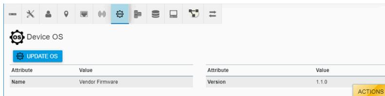
The storage **Device OS** section displays the device's firmware version and can be used to upgrade firmware.
