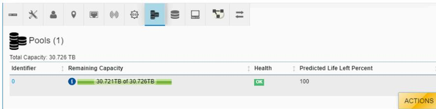
The storage device's **Pools** section shows all of the pools configured on the storage device. The number of pools can be set to 1, 2, 4, or 8.
