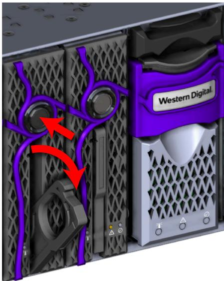
**Figure 263:** OpenFlex F3x00 Release Operation
