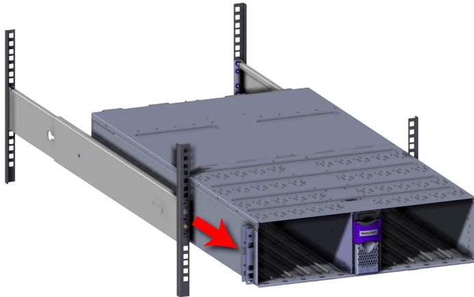
**Step 6:** Remove the Rack Mount Rails.
