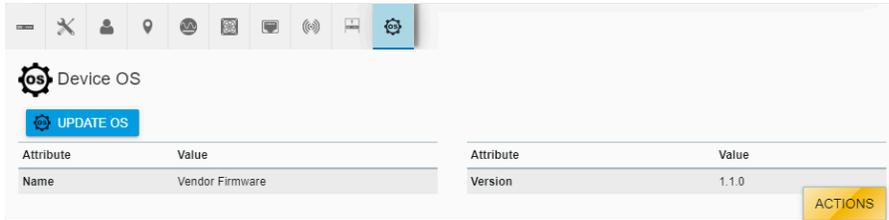
The chassis's **Device OS** section displays the firmware version and can be used to upgrade firmware.
