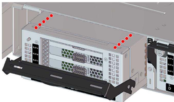
**Step 8:** Uninstall the remaining IO Module (IOM) in the same way the first was uninstalled.
