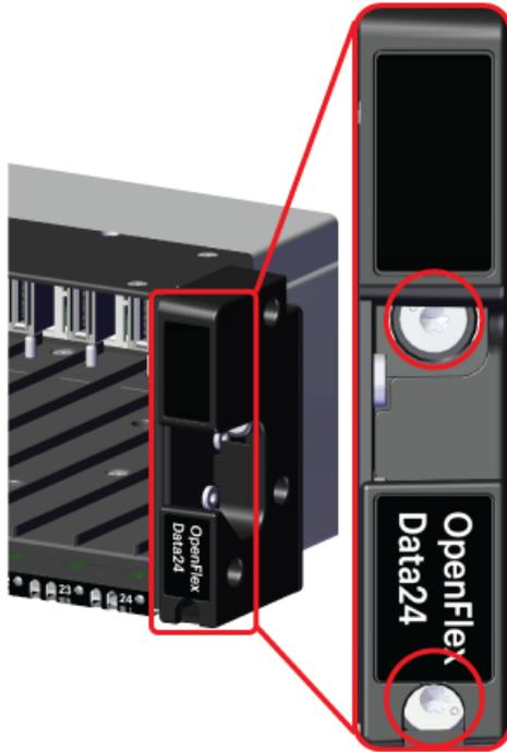
**Step 14:** Install the Drive Assembly into the enclosure.
