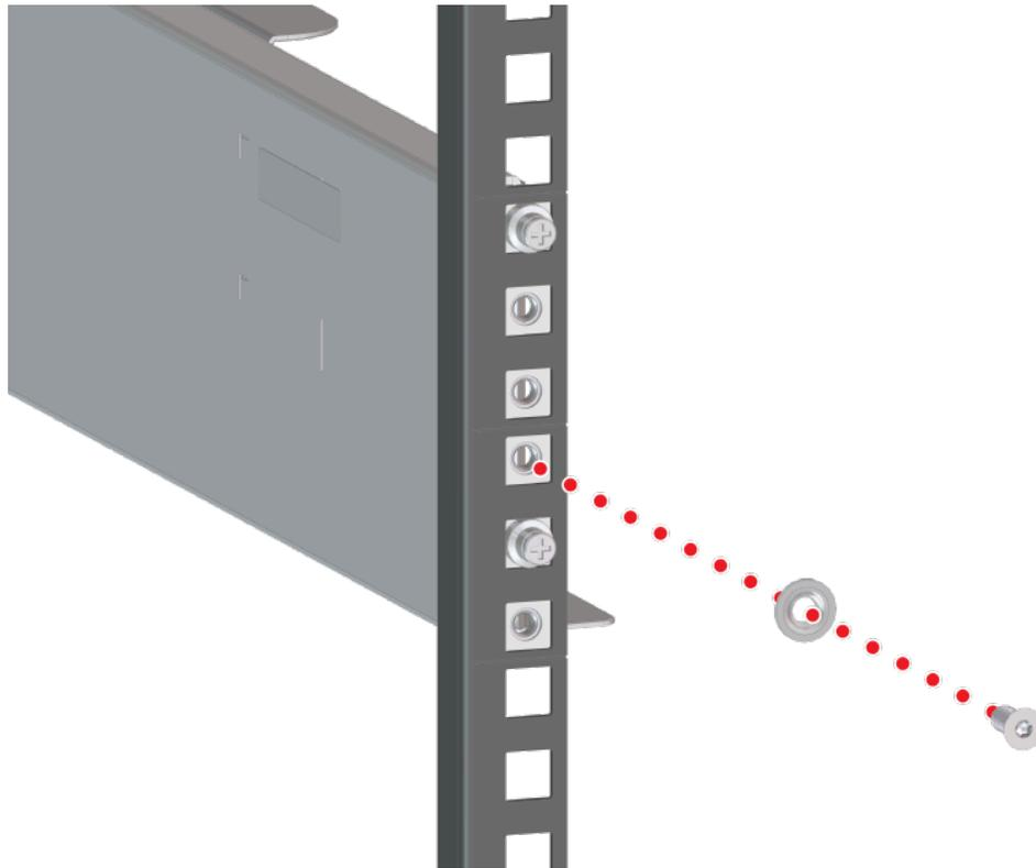
**Step 9:** Install the remaining Rails in the same way the first was installed.
