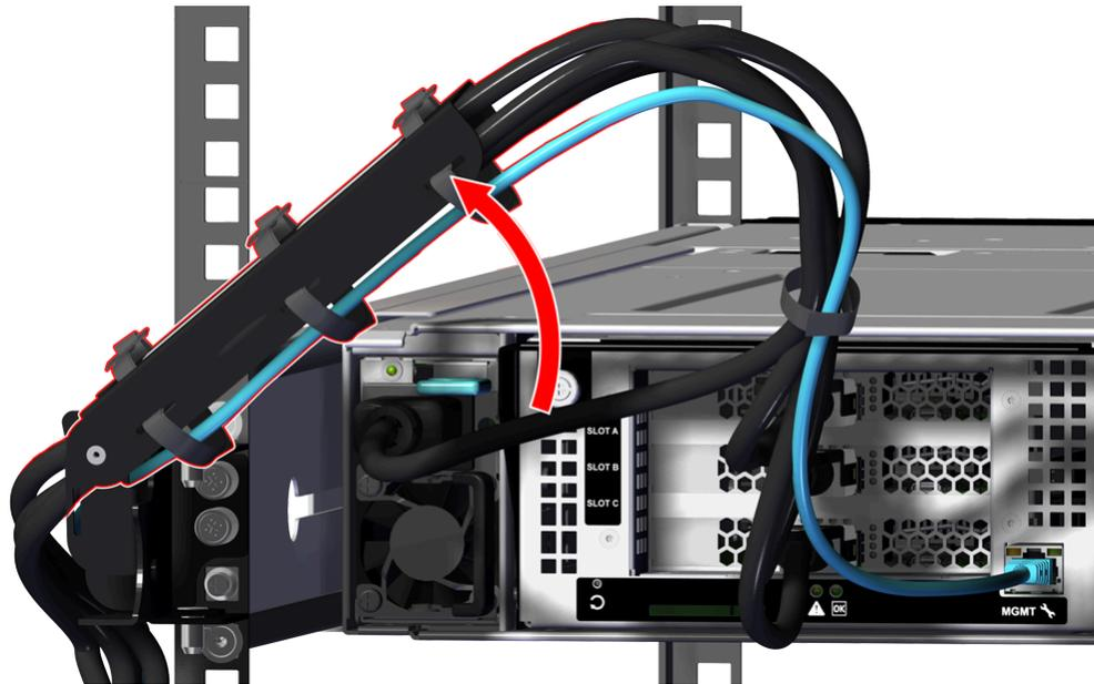
**Step 3:** Uninstall the Power Supply Unit (PSU) from the enclosure.
