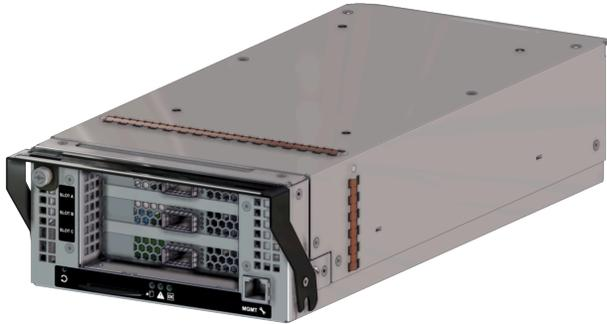
Each IOM provides system data connectivity through up to three QSFP28 cables per IOM, and supports cable lengths up to 10m. Out-of-Band Management (OOBM) features are accessed via an RJ45 port that supports a 10/100/1000 Mbps Ethernet connection. The IOM status LEDs report Fault and Power. The IOM is hotswappable and easily removable by removing cables/connectors, loosening the single thumbscrew and pulling on the handle.
