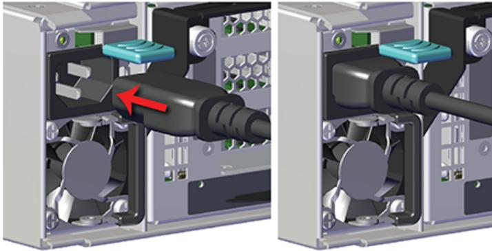
*Figure 60: Locking the Retention Clip*
