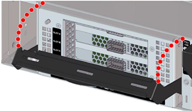
Figure 45: Uninstall IO Module (IOM)
