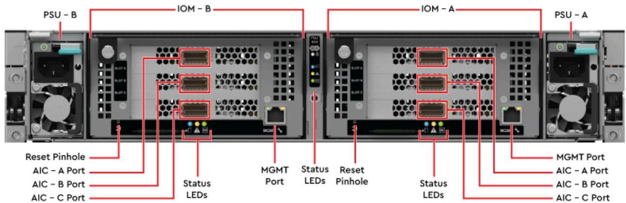
Each IOM contains a Reset Pinhole that will factory reset the enclosure if it is pressed for more than three seconds. The enclosure automatically restarts when the reset completes. Use of the Reset Pinhole is not recommended in Low Power Mode. Both of the systems IOMs will be factory reset when initiating the reset using the Reset Pinhole on a single IOM.
