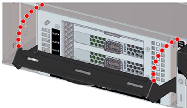
Figure 75: Uninstall IO Module (IOM)
