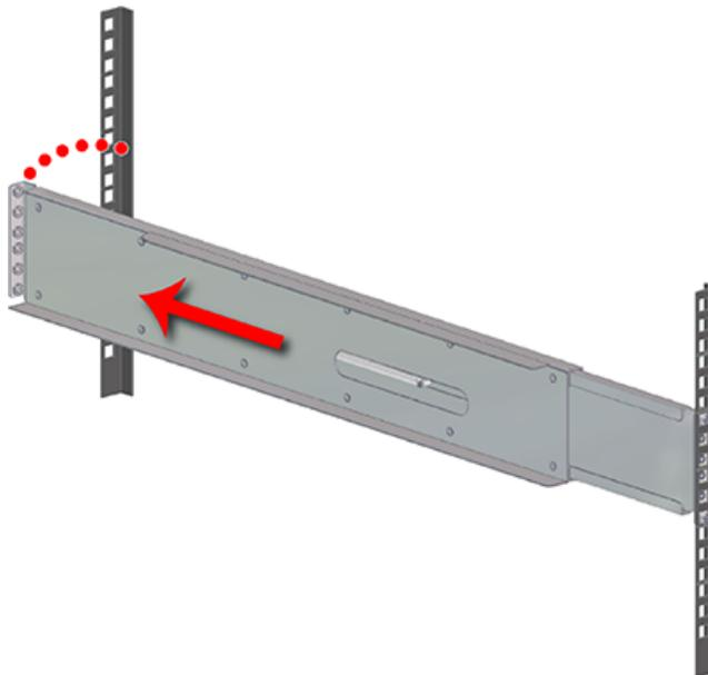
**Step 6:** Uninstall the remaining Rails in the same way the first was uninstalled.
