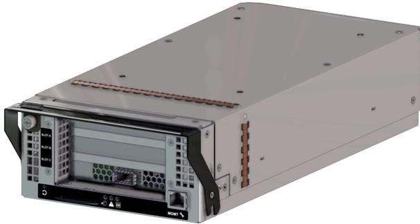
Each IOM provides system data connectivity through a QSFP28 cable, and supports cable lengths up to 10m. Out-of-Band Management (OOBM) features are accessed via an RJ45 port that supports a 10/100/1000 Mbps Ethernet connection. The IOM status LEDs report Fault and Power. The IOM is hotswappable and easily removable by removing cables/connectors, loosening the single thumbscrew and pulling on the handle.
