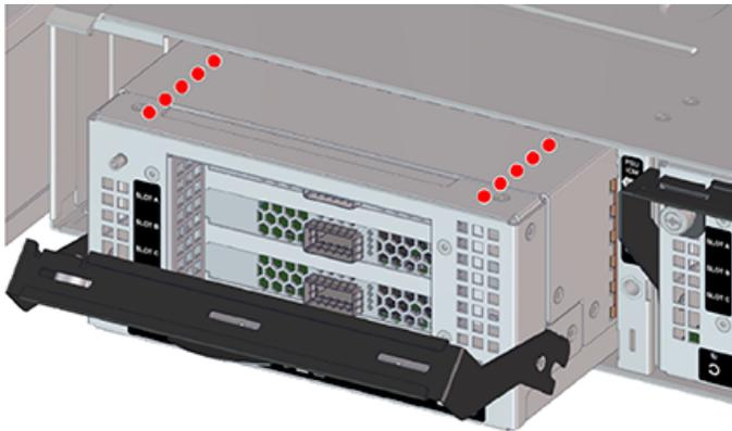
**Step 4:** Unpack and inspect the new IO Module (IOM) for damage.
