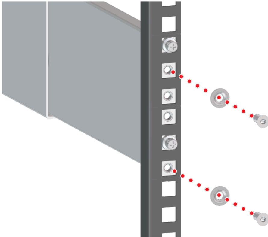
*Figure 113: Remove Rail*
