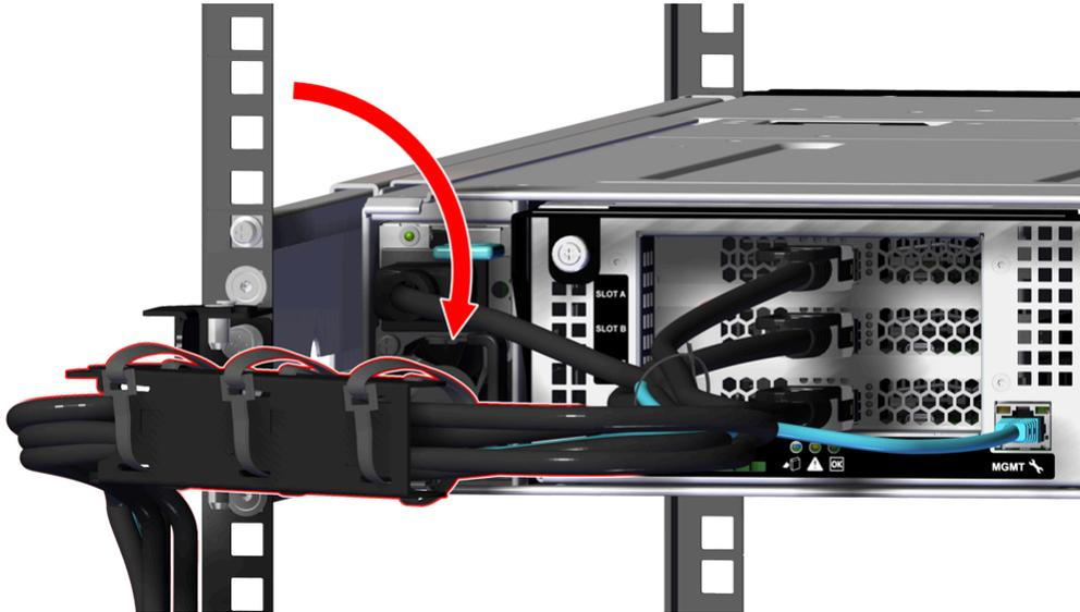
**Step 22: (Optional)** Repeat the previous step to return the remaining arm to the operational state.
