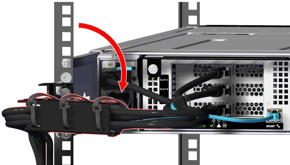
**Step 7:** Connect the power cable to the Power Supply Unit (PSU) and loop the PSU's retention clip around the power cable and pinch it until the clip catches and locks in place.
