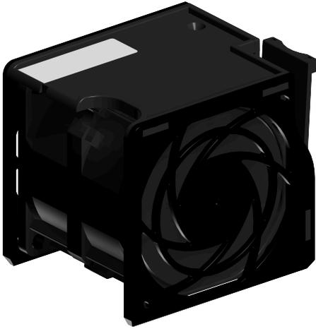
The system fans provide the primary system cooling for the OpenFlex Data24. There are a total of five N+1 redundant fans, and they are accessible from a latch cover on the top of the chassis. The system fans are hot swappable CRU components, and do not require any wiring. The plastic fan covers also have labels identifying each fan.
