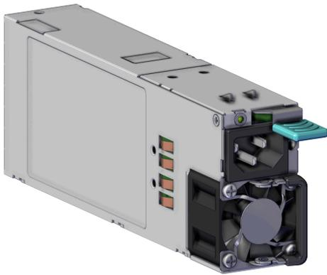
The Gospower Power Supply Unit (PSU) inside the OpenFlex Data24 are 2000W, 80 Plus Titanium efficiency rated, and operate within a 200 - 240 VAC voltage range. The PSUs are redundant and can be hot swapped one at a time. There must always be one PSU in operation for continuous usage during replacements of the PSUs.
