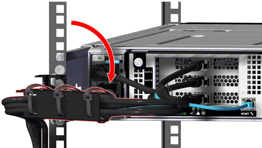
**Step 14: (Optional)** Repeat the previous step to return the remaining arm to the operational state.
