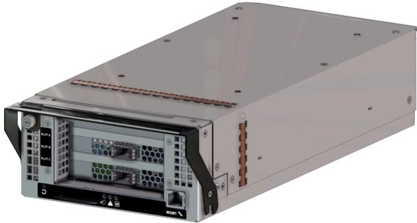
Each IOM provides system data connectivity through up to two QSFP28 cables per IOM, and supports cable lengths up to 10m. Out-of-Band Management (OOBM) features are accessed via an RJ45 port that supports a 10/100/1000 Mbps Ethernet connection. The IOM status LEDs report Fault and Power. The IOM is hotswappable and easily removable by removing cables/connectors, loosening the single thumbscrew and pulling on the handle.
