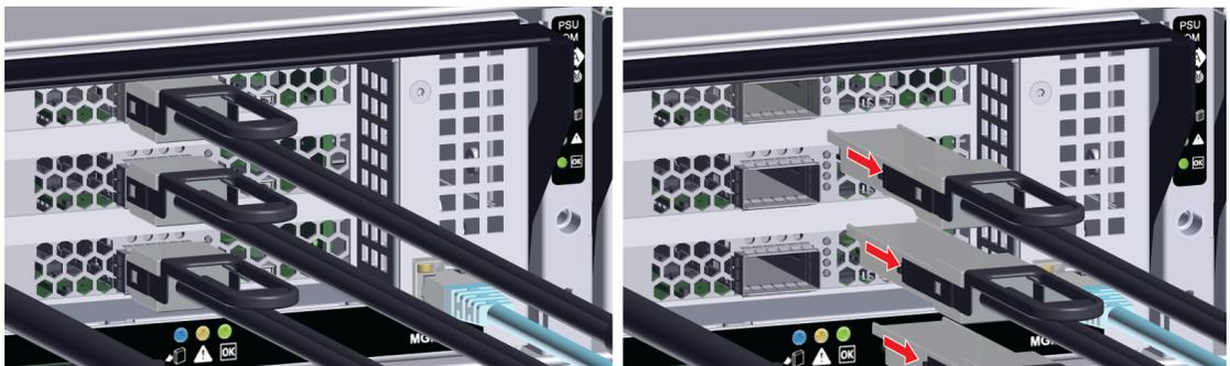
**Step 2: (Optional)** If your configuration contains a CMA, carefully move the arm on the side in need of servicing away from the system. This will allow for ease of access to the components on the chosen side while keeping the system cabling organized and safe. The CMA must be removed before attempting to remove the rails.
