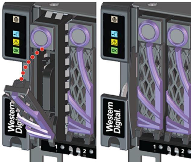
**Step 15:** Install the remaining Drive Assembly in the same way the first was installed.
