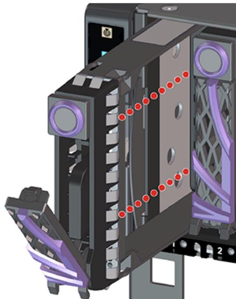
**Step 10:** Uninstall each Drive Assembly in the same way the first was uninstalled.
