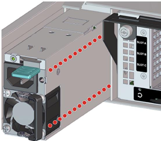
**Step 6:** Uninstall the remaining Power Supply Unit (PSU) in the same way the first was uninstalled.
