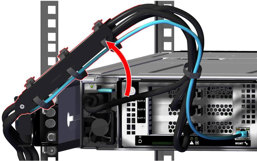
**Step 3: (Optional)** Repeat the previous step to move the remaining arm into the servicing state.
