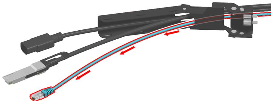
**Step 10:** Repeat the previous step to install the cables into remaining CMA.
