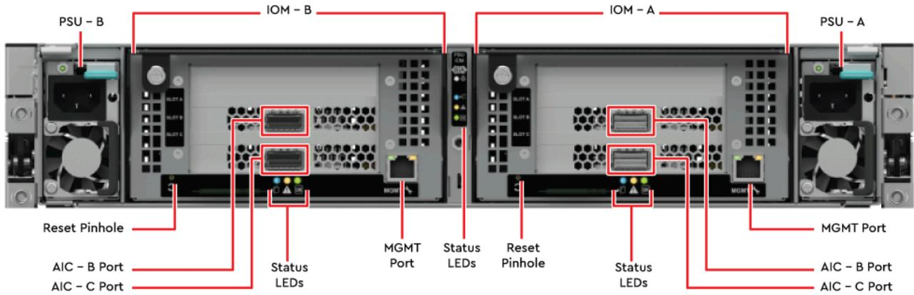
Figure 5: Three AIC Configuration
