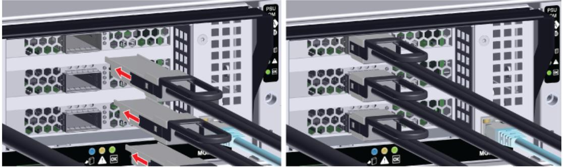
**Result:** The IO Module (IOM) has now been replaced.
