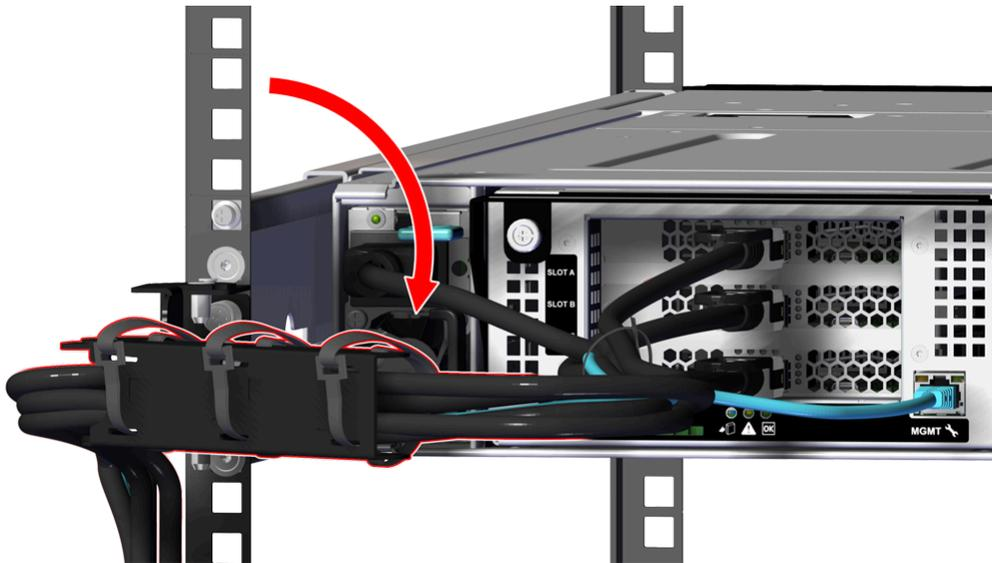
**Step 7:** Connect the data cables to the IO Module (IOM).
