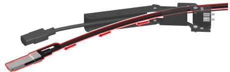
c. Route the Management cable through the channel in the CMA until about 18 in on the cable is sticking out of the other end. The amount of cable slack can be adjusted once the CMA is installed.
