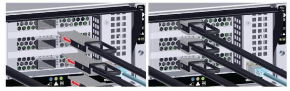
Result: The IO Module (IOM) has now been replaced.
