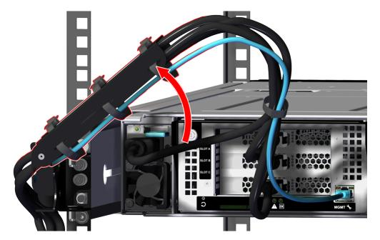
Figure 65: Move CMA Assembly into a Servicing State
