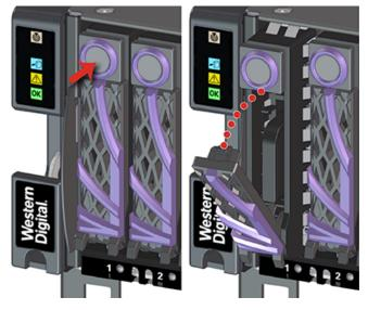
**b.** Use the release handle to pull the Drive Assembly out of the enclosure.
