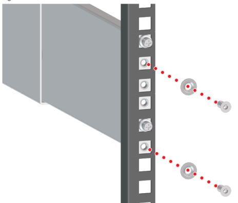
Figure 116: Install Rear Rack Mount
