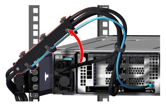
Figure 53: Move CMA Assembly into a Servicing State
