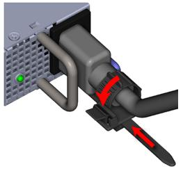
**f.** Slide the retention clip forward until it stops near the cable connector. Doing this will ensure that the retention clip functions properly in the event the cable is accidentally pulled.
