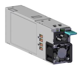
The Gospower Power Supply Unit (PSU) inside the OpenFlex Data24 are 2000W, 80 Plus Titanium efficiency rated, and operate within a 200 - 240 VAC voltage range. The PSUs are redundant and can be hot swapped one at a time. There must always be one PSU in operation for continuous usage during replacements of the PSUs.
