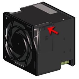
**d.** Carefully pull the System Fan out of the System Fan slot.
