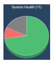
The **System Health** section provides an overview of the health of the fabric network. The interfaces of all devices on the same subnet as the Storage devices are queried when the page loads, and the pie chart is updated with their responses. If fabric devices respond with errors or faults, the system health chart will update accordingly.
