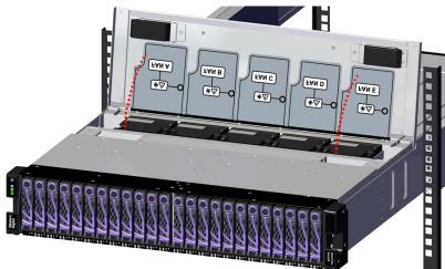
**c.** Grasp the System Fan firmly with your index finger, and use your thumb to press the latch release using a pinching motion.
