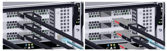
**Step 2:** If your configuration contains a CMA, carefully move the arm on the side in need of servicing away from the system. This will allow for ease of access to the components on the chosen side while keeping the system cabling organized and safe. The CMA must be removed before attempting to remove the rails.
