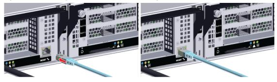
**b.** Connect the QSFP28 cables into all of the IOM ports.
