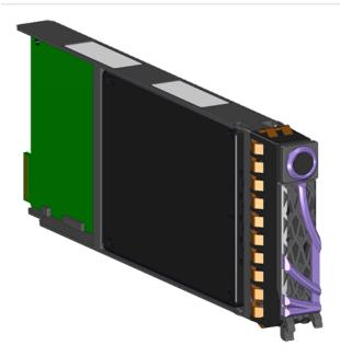
The drive assembly is comprised of 3 basic parts: the 2.5 in. SSD, the drive carrier, and the active interposer card. The drive carrier houses the 2.5 in. drive and the interposer card and enables toolless installation and replacement. The drive assembly is available in many different volumes, encryption, and block sizes.
