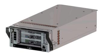
Each IOM provides system data connectivity through up to three QSFP28 cables per IOM, and supports cable lengths up to 10m. Out-of-Band Management (OOBM) features are accessed via an RJ45 port that supports a 10/100/1000 Mbps Ethernet connection. The IOM status LEDs report Fault and Power. The IOM is hotswappable and easily removable by removing cables/connectors, loosening the single thumbscrew and pulling on the handle.
