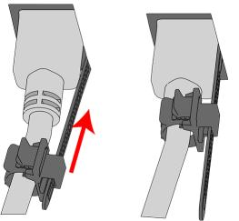
Figure 126: Sliding the Retention Clip Forward
