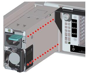
Figure 72: Uninstall Power Supply Unit (PSU)
