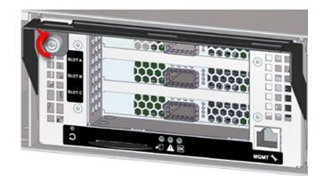
**d.** Verify that the IO Module (IOM) is securely latched into the Chassis by pulling on the release handle and ensuring the IO Module (IOM) does not move when pulled. Reinstall the IO Module (IOM) if it is not securely installed into the Chassis.
