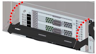
Figure 45: Uninstall IO Module (IOM)
