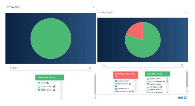
The **Storage Health** modal provides an overview of the health of all storage devices visible on the fabric (those in the subnets of what is configured on the enclosure). The modal provides separate tables for fabric devices that are presenting different health states up to the OCGUI.
