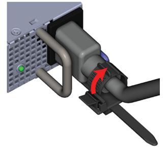
d. Connect the power cables into the two Power Supply Unit (PSU) power connectors.
