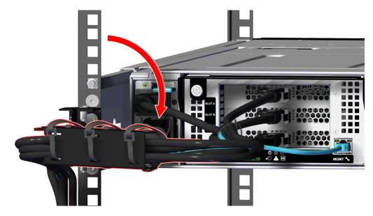
Figure 96: Return the CMA Assembly to the Operational State
