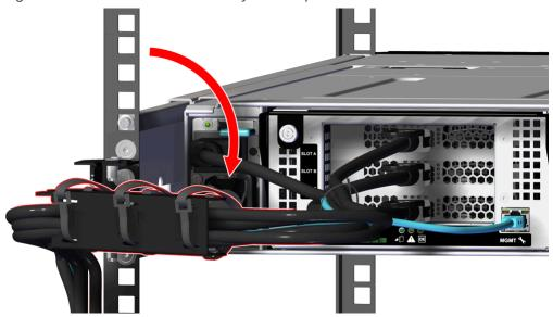
Figure 140: Return the CMA Assembly to the Operational State
