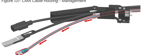
Figure 137: CMA Cable Routing - Management
