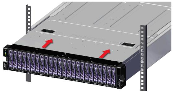
**b.** Using the T15 Torx screwdriver, tighten the two Torx captive screws, located under the rack ear cutouts, to secure the Chassis to the rail. Repeat this step to secure the remaining rack mount to the remaining rail.
