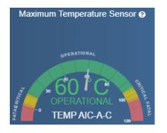
The storage **Maximum Temperature Sensor** section provides a visual summary of the current Maximum Temperature of the device. When the Maximum Temperature Sensor is selected it will display the device with the highest temperature.
