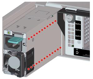
**b.** Verify that the Power Supply Unit (PSU) is fully seated and latched into the Power Supply Unit (PSU) slot by gently pulling on the handle.
