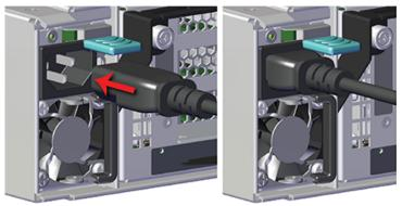
Figure 60: Locking the Retention Clip
