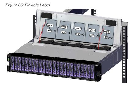
c. Grasp the System Fan firmly with your index finger, and use your thumb to press the latch release using a pinching motion.
