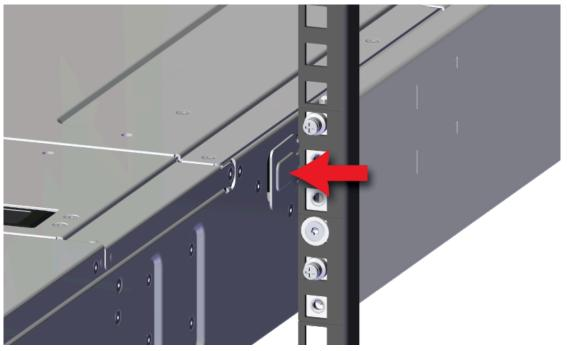
**d.** Continue sliding the chassis out of the rack and ensure extra care is taken to support the weight of the Chassis when the Chassis is clear of the rack mount rails.
