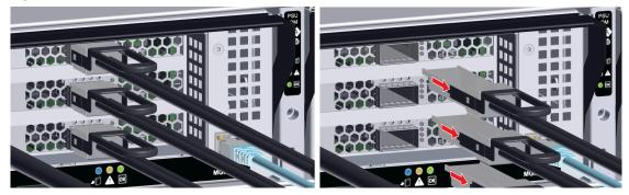
**Step 2: (Optional)** If your configuration contains a CMA, carefully move the arm on the side in need of servicing away from the system. This will allow for ease of access to the components on the chosen side while keeping the system cabling organized and safe. The CMA must be removed before attempting to remove the rails.
