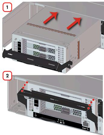
Figure 47: IO Module (IOM) Handle Engaged
