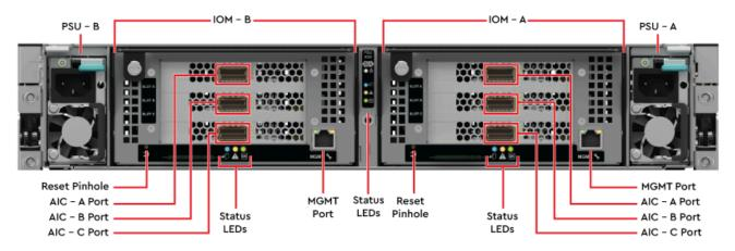
Each IOM contains a Reset Pinhole that will factory reset the enclosure if it is pressed for more than three seconds. The enclosure automatically restarts when the reset completes. Use of the Reset Pinhole is not recommended in Low Power Mode. Both of the systems IOMs will be factory reset when initiating the reset using the Reset Pinhole on a single IOM.
