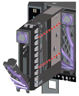
Step 10: Uninstall each Drive Assembly in the same way the first was uninstalled.
