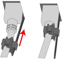
Figure 102: Sliding the Retention Clip Forward
