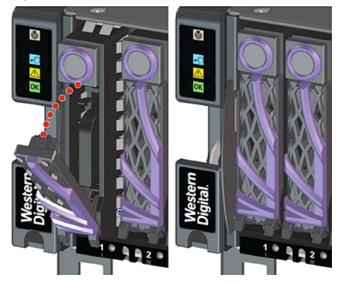
Figure 85: Drive Assembly Installation
