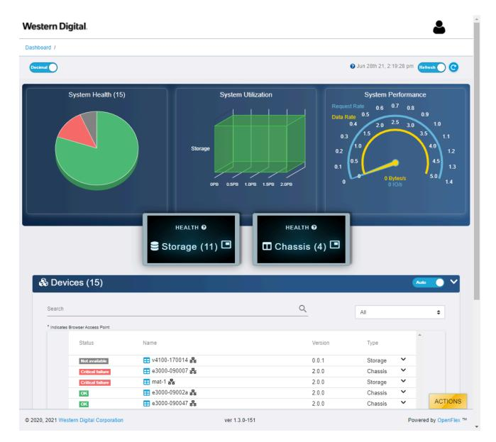
The **Dashboard** is the first page that will load when one logs into **any** of the fabric-attached devices. It provides vital statistics on the health and performance of all devices on the subnet configured on the Enclosure Manager. In addition, it provides a clickable list that allows users to navigate to the device page for any device on the subnet.
