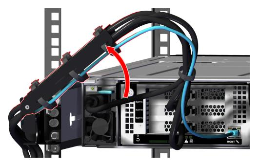
Figure 131: Move CMA Assembly into a Servicing State
