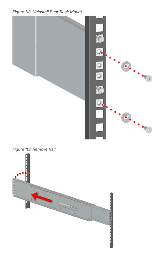
Step 6: Uninstall the remaining Rails in the same way the first was uninstalled.Step 7: Unpack and inspect the new Rails for damage.
