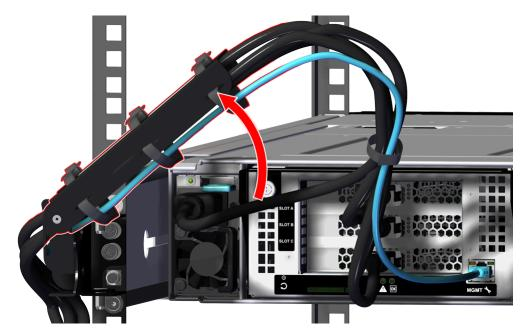
Figure 107: Move CMA Assembly into a Servicing State
