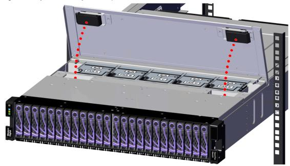
Figure 37: System Fan Bay Cover Operation
