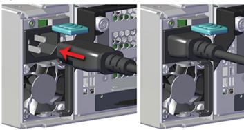
Figure 124: Connect Power Cables
