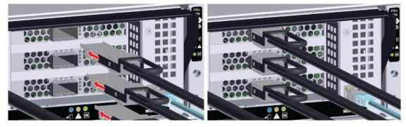
c. Unclip the retention strap on the PSU as shown in the following image.
