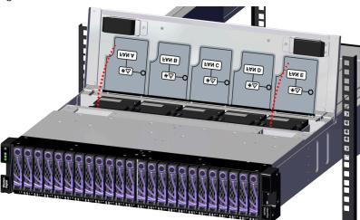
**c.** Orient the System Fan with the module latch (and connector) on the right-hand side and insert it into the System Fan slot.
