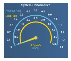
The **System Performance** section provides general, bitwise system performance information for all devices on the fabric. The GUI contains a System Performance gauge, but it will not provide performance for Data24. Other Systems may display performance using this gauge. Data24 can display performance using Linux specific monitoring like **iostat**.
