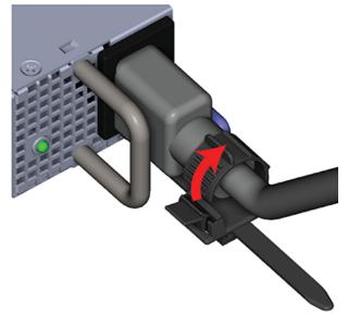
b. Disconnect the power cables from each of the two Power Supply Unit (PSU).
