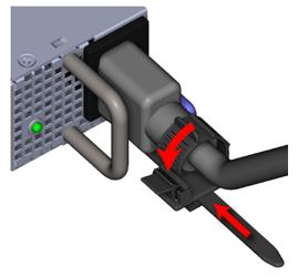
**f.** Slide the retention clip forward until it stops near the cable connector. Doing this will ensure that the retention clip functions properly in the event the cable is accidentally pulled.
