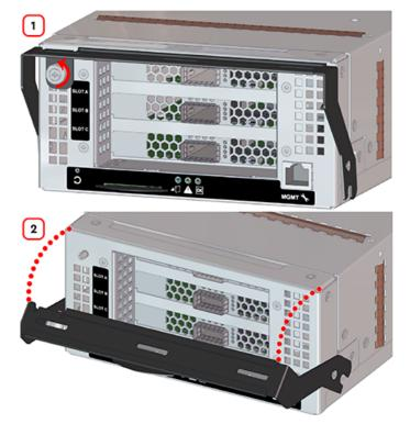
**b.** Gently slide the IO Module (IOM) into the IO Module (IOM) slot until the release handle is engaged with the Chassis. When the handle lifts up slightly, it is an indicator that the release handle is engaged with the Chassis.
