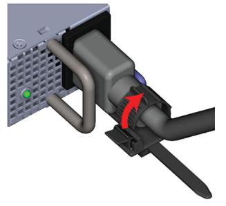
b. Disconnect the power cables from each of the two Power Supply Unit (PSU).
