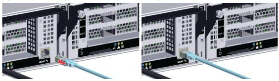
b. Connect the QSFP28 cables into all of the IOM ports.
