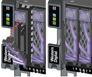
**Result:** The Drive Assembly has now been replaced.
