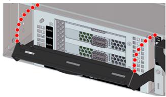
Figure 74: IO Module (IOM) Release Handle Operation
