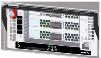
Figure 43: IO Module (IOM) Thumbscrew Operation
