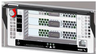
Figure 73: IO Module (IOM) Thumbscrew Operation
