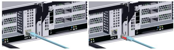
**b.** Disconnect the QSFP28 cables from all of the IOM ports.
