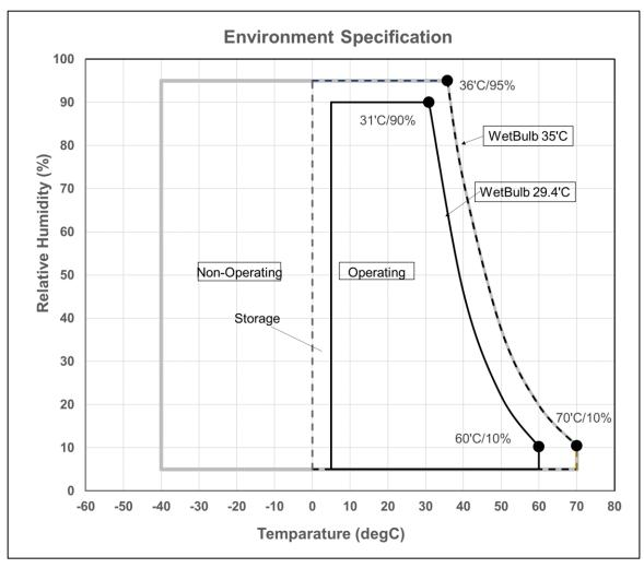
Figure 5 Limits of temperature and humidity
