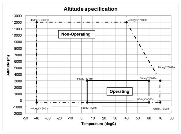
Figure 4 Limits of temperature and altitude
