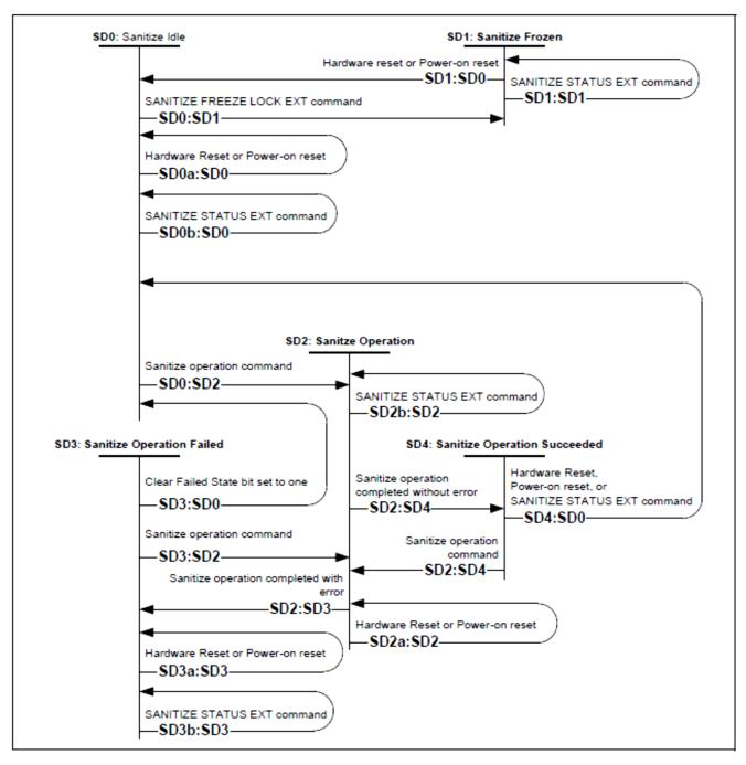
Figure 12 Sanitize Device state machines
