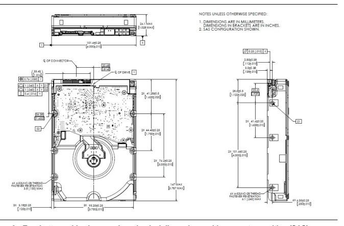
Figure 9 Top, bottom, side views, and mechanical dimensions, with connector position (SAS) All dimensions in the above figure are in millimeters.
