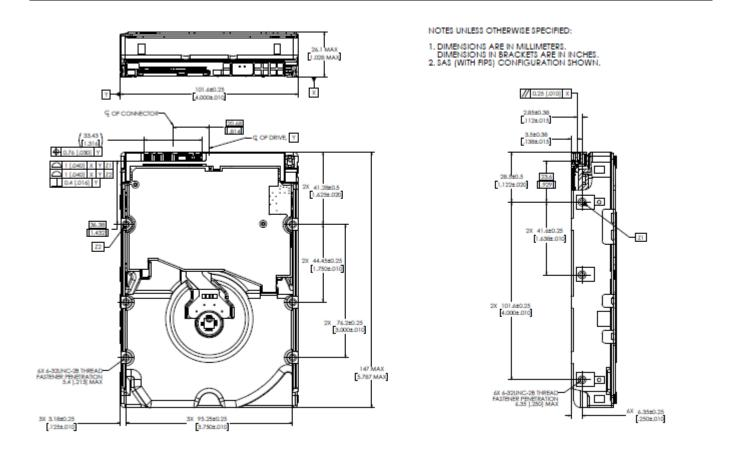
Figure 10 Top, bottom, side views, and mechanical dimensions, with connector position (FIPS model)
