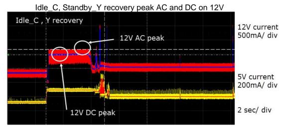
Figure 7 Idle\_C Standby\_Y recovery current waveform
