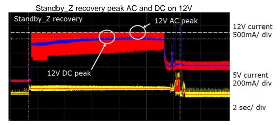
Figure 8 Standby\_Z recovery current waveform
