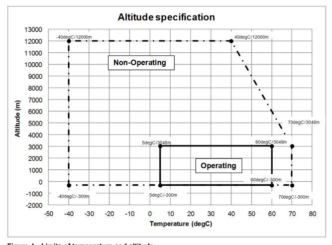
Figure 4 Limits of temperature and altitude
