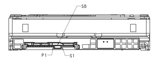
Figure 3 Connector pin assignments
