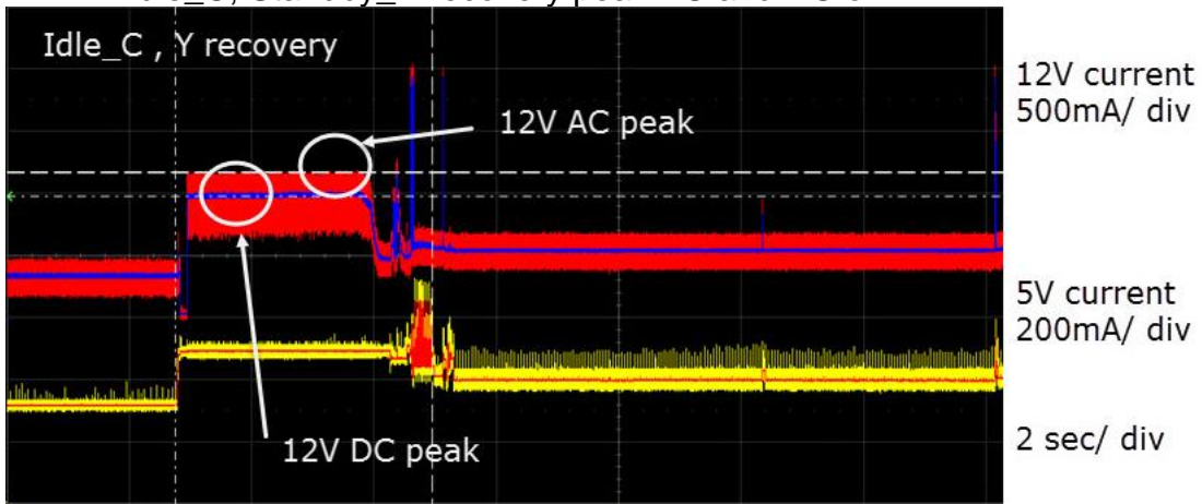
Figure 7 Idle_C Standby_Y recovery current waveform
