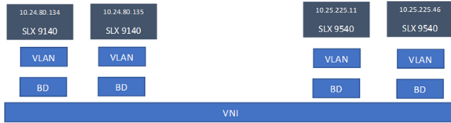
Figure 18: Scope of tenant constructs
