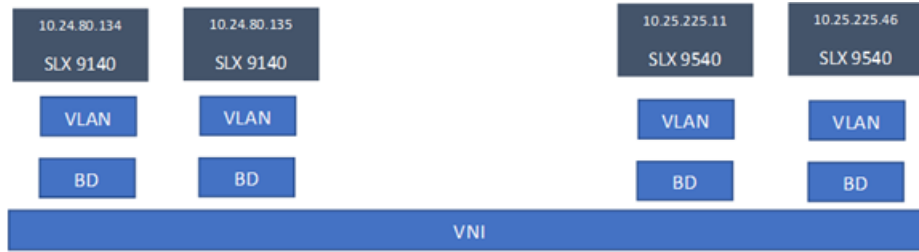
Figure 18: Scope of tenant constructs
