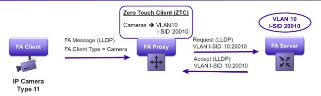
Figure 39 FA Zero-Touch-Client Assigns VLAN:I-SID Binding to Discovered FA client
