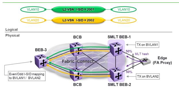
Figure 90 L2 VSN Load Balancing into SPB Equal Cost Shortest Paths
