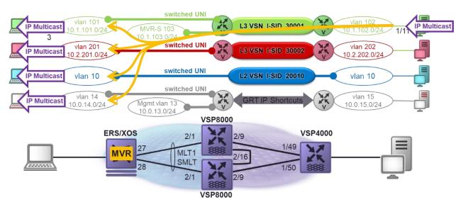
Figure 49 Inter-VSN IP Multicast with MVR on FA Proxy
