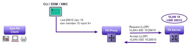
Figure 41 VLAN:I-SID Binding via Manual Configuration
