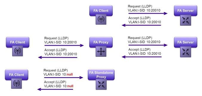
Figure 35 Fabric Attach Model
