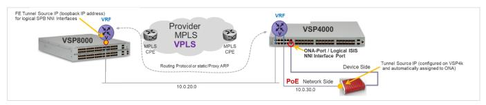
Figure 59 Fabric Extend Deployment Model over WAN L2 E-LAN Service
