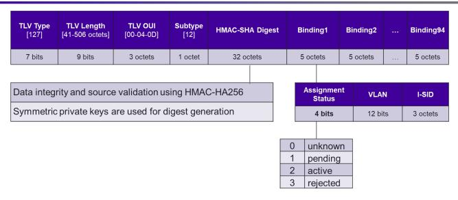
Figure 37 Fabric Attach LLDP Service Signalling TLV
