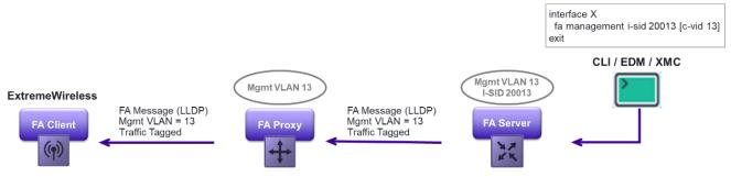
Figure 44 FA Signalling of Management VLAN from FA Server
