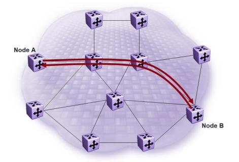
Figure 18 Unicast Shortest Path Between Two Nodes; Forward & Reverse Congruent
