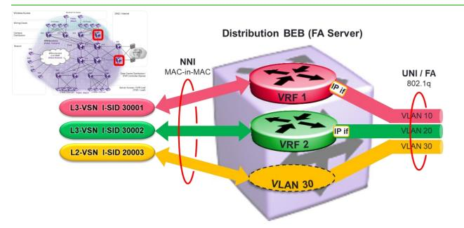
Figure 81 Zoom on Distribution BEB with UNI/FA Interfaces
