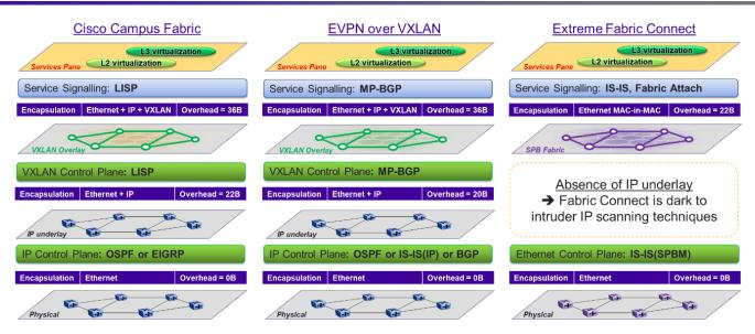
Figure 6 Overview of Fabric Layers and Overlays
