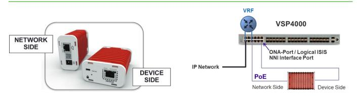
Figure 52 Fabric Extend Pairing of ONA with VSP4000
