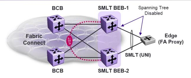
Figure 86 Split Multi-Link Trunking (SMLT) Used in SPB Fabric Access
