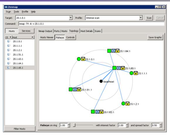
Figure 95 L3 VSN Topology as Seen by IP Scanning Tools
