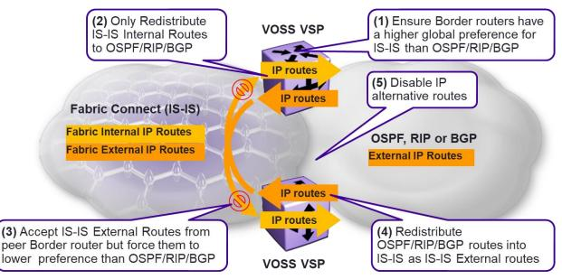
Figure 28 Redundantly IP Routing Fabric VSN with External OSPF/RIP/BGP Network
