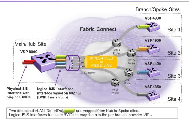
Figure 60 Fabric Extend over WAN L2 Point-to-Point E-LINE Services
