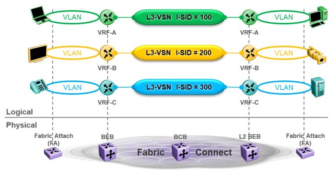
Figure 3 Virtualization with SPB L3 VSNs
