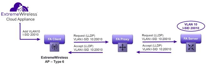
Figure 38 FA Client Requests VLAN:I-SID Binding
