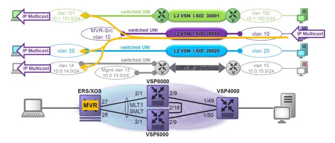
Figure 50 Inter-VSN IP Multicast with Fabric-wide MVR L2 VSN
