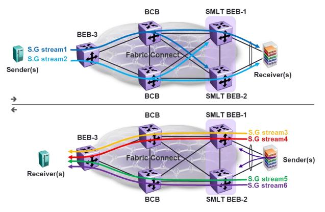
Figure 91 IP Multicast Load Balancing into SPB Equal Cost Shortest Path Trees
