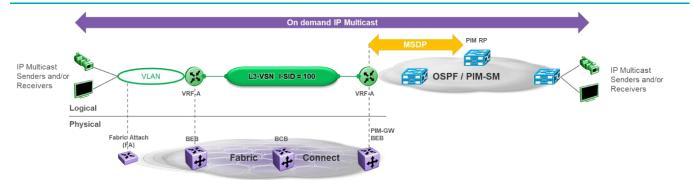
Figure 47 PIM Gateway to Legacy IP Multicast Routed Networks
