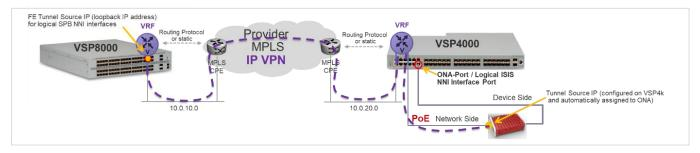
Figure 55 Fabric Extend Deployment Model over WAN L3 IPVPN Service
