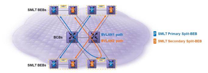
Figure 22 SPB shortest path optimization via SMLT Primary/Secondary BEB positioning
