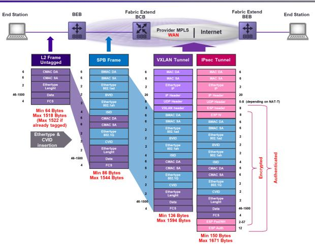
Figure 53 Fabric Extend IP Mode (VXLAN / IPsec) MTU Considerations
