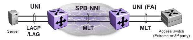
Figure 85 Multi-Link Trunking (MLT) Used in Core and Access
