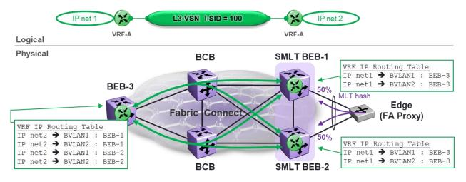
Figure 89 L3 ECMP Translation into SPB Equal Cost Shortest Paths
