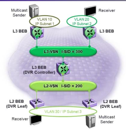
Figure 46 IP Multicast Over L3 VSN that Comprises L2 VSNs
