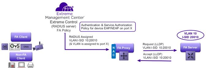
Figure 40 VLAN:I-SID Binding is RADIUS Assigned via NAC
