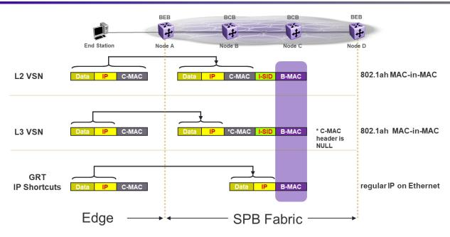
Figure 23 Different Encapsulation Used by GRT IP Shortcuts
