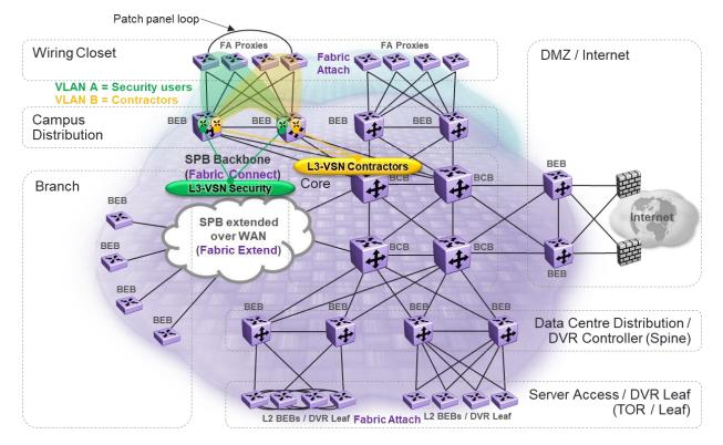
Figure 93 Access VLANs Collapsed Together
