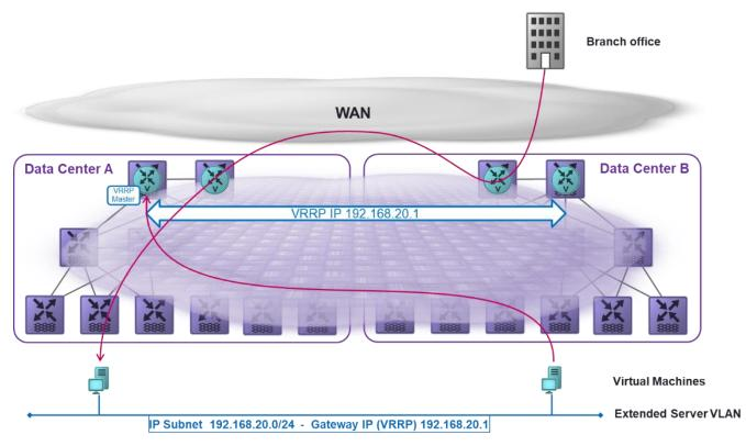
Figure 64 Traffic Tromboning Challenges in a Non-DVR Enabled Data Center
