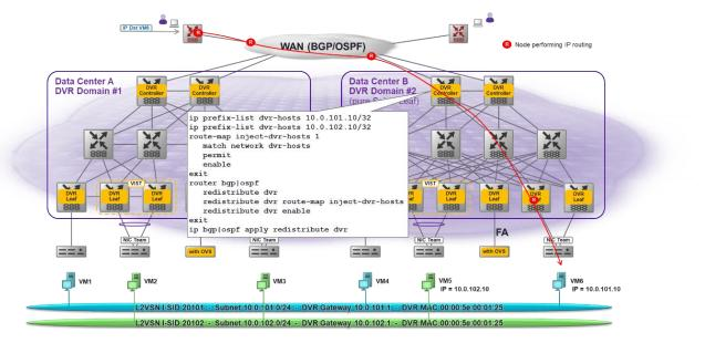
Figure 74 Eliminating North-South Tromboning with DVR, Over Legacy WAN
