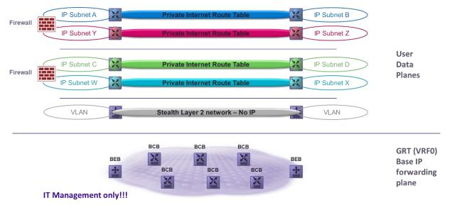
Figure 96 Isolation of the Global Routing Table (VRFO)
