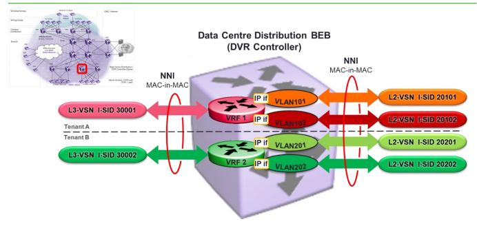
Figure 83 Zoom on Data Center Distribution BEB / DVR Controller
