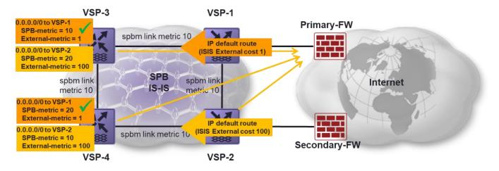
Figure 27 IS-IS External Routes Prefer Lower Route Metric over SPB's Shortest Path
