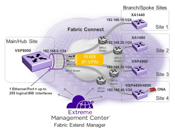
Figure 54 Fabric Extend over WAN L3 Any-to-Any IPVPN Service
