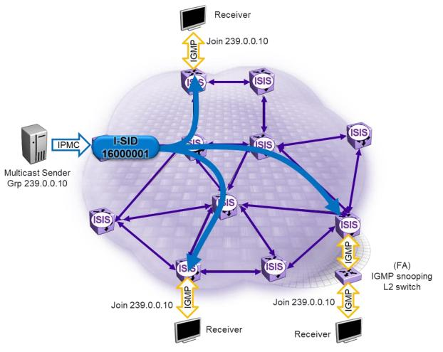
Figure 45 IP Multicast with SPB
