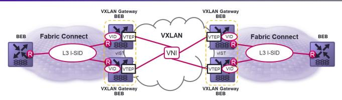
Figure 63 Extending an L3 VSN across Fabrics with VXLAN Gateway
