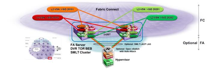
Figure 84 Data Center Top of Rack (ToR) BEB with SMLT clustering
