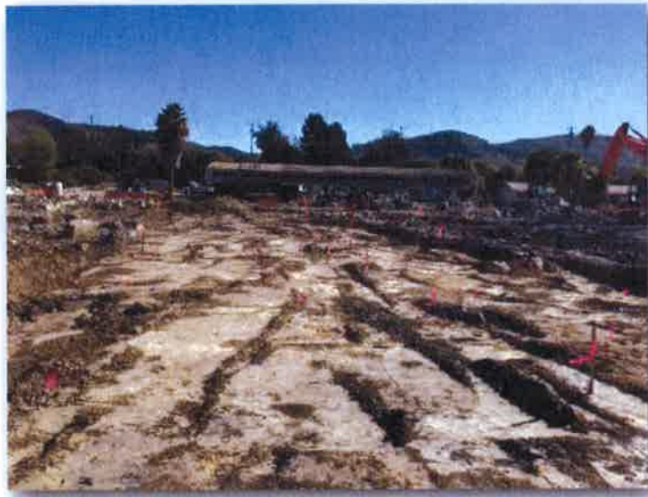
Typical Perimeter Sampling Grid in Former Asphalt Covered Area (Approx. 1' Below Grade)
