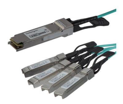
The QSFP4X10GAO5 is a Cisco QSFP-4X10G-AOC5M compatible optical quad small form-factor pluggable (QSFP+) breakout cable that is designed, programmed and tested to work with Cisco® brand compatible servers or routers and complies with MSA industry standards. Connecting a single QSFP+ port (40 GbE) to four 10G SFP+ ports, this active optical breakout cable is fully hot-pluggable which makes upgrades and replacements seamless by minimizing network disruptions.
