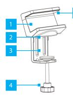
Slide the Device (e.g. Power Strip) into the Adjustable Clamp, securing the Device in place. The Power Strip Desk Clamp will adjust to the size of the Device, between 40 mm - 60 mm (1.6" - 2.4") wide.
