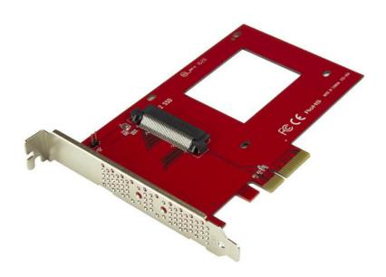
Get ultra-fast data access by adding an NVMe U.2 SSD to your computer. This U.2 to PCIe adapter lets you add a high-speed, U.2 (4-lane PCIe) 2.5" NVMe SSD, such as the Intel® 750 Series drive, to a PC with an available x4 PCI Express expansion slot.
