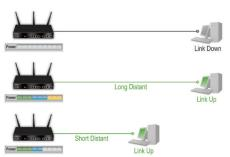
The D-Link Green Ethernet power-saving program can adjust power by detecting link status and cable length.
