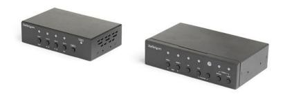
This multi-input HDBaseT<sup>M</sup> extender kit extends your A/V signals to a remote location up to 230 ft. (70 m) away. It features a built-in switch and scaler, so you can choose which video source is output from four independent video sources (2 x HDMI, 1 x VGA and 1 x DisplayPort).
