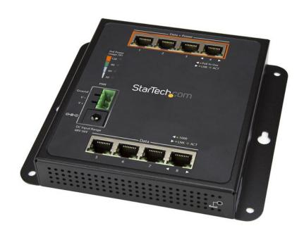
Easily deploy or scale your network with this Gigabit Ethernet switch, by adding eight copper Gigabit Ethernet (GbE) connections, including four PoE+ ports. This IP30 industrial network switch provides intelligent Layer 2 management. Its rugged, compact design and wall-mount option with front access make it ideal for demanding applications, even where space is limited.
