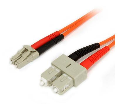
The FIBLCSC2 2-meter (6.6ft) Multimode 62.5/125 Duplex Fiber Patch Cable is terminated with one LC (male) connector and one SC (male) connector, to provide the necessary connection between fiber networking devices for high-speed, long distance networks.
