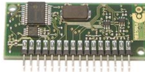
Figure 13: Receiver devices RCM 110 and RCM 120
