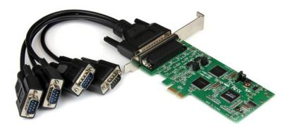
The PEX4S232485 4 Port PCI Express PCIe Serial Combo Card - 2 x RS232 2 x RS422 / RS485 lets you add two RS232, and two RS422/485 serial ports to your PC through a PCI-Express expansion slot.
