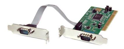
This 2 Port 16550 Serial Card can be installed in a PCI slot to add two serial ports - a cost-effective solution for connecting any new serial device or old legacy serial device, with data transfer rates of up to 115.2 Kbps. The serial card features a low profile bracket, suitable for installation in low profile/small form factor computer cases.
