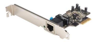
This PCI Express based 10/100 Ethernet Card provides a simple way to connect a PCIe enabled server or workstation to a 10/100 Ethernet network and offers a broad range of features and functions, including support for both Full and Half Duplex operation as well as Wake On LAN (WOL) Power Management.
