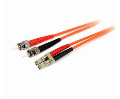
The FIBLCST2, 2-meter (6.6ft) Multimode 62.5/125 Duplex Fiber Patch Cable is terminated with one LC (male) connector and one ST (male) connector, to provide the necessary connection between fiber networking devices for high-speed, long distance networks.
