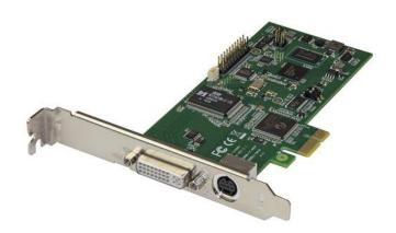
This PCIe video capture card lets you record 1080p HD video and 2-channel stereo audio (HDMI/RCA) to your computer system. With multiple video inputs, including HDMI, DVI, VGA and component, this all-in-one capture card can record original content from virtually any device.
