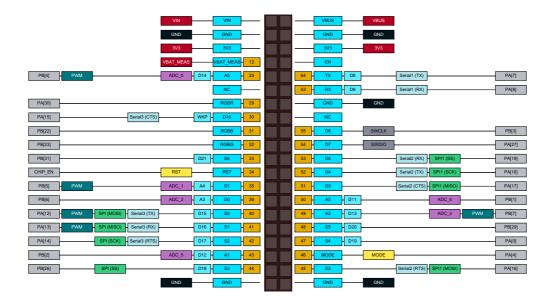
See the P2 Datasheet for details about the pins. The gold boxes indicate the P2 pin numbers.
