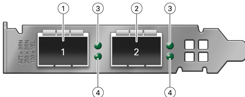
**Note** - If your adapter is installed horizontally, the ports are numbered 1 and 2, left to right. In a vertical orientation, the ports are numbered 1-2 bottom to top.
