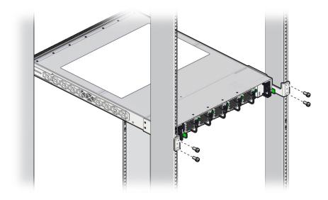
8. If you are using the CMA, attach the CMA bracket and CMA cover to the short rail brackets using the outer green thumbscrews.
