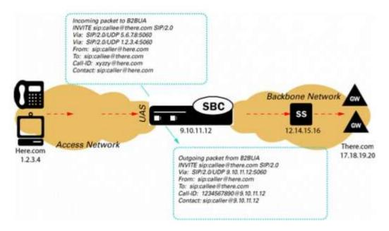
In an access model the SBC is contacted by a SIP endpoint to relay endpoint signaling information. The IP address of the endpoint is usually not known, so trust should be established through behavior such as establishment of a successful registration. Once the endpoint becomes trusted, dynamic Access Control Lists (ACL) and Call Admission Controls (CAC) can be applied. Monitoring of potentially abusive behaviors provides a mechanism to "demote" or blacklist endpoints.
