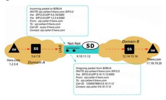
In a peering model the SBC is contacted by a SIP server to relay endpoint signaling information. The SIP server may be a PBX, registrar, proxy, SBC, or other device. The IP of the device is usually trusted and pre-provisioned in the SBC as an endpoint (session agent) that will be relaying calls. Since the remote endpoint is already known, Access Control Lists (ACL) and Call Admission Controls (CAC) can be pre-provisioned for the appropriate level of protection or service level assurance.
