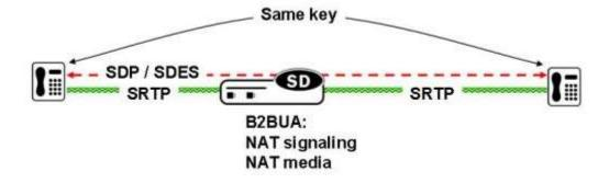
If the configuration specifies "pass-through" mode, the SBC will not intercept the crypto attribute exchange between the caller and the callee. The crypto attribute will be forwarded as it is from the caller to the callee and vice versa.
