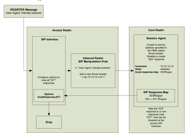
Some customers have asked about using the "reject" action in HMRs to send a "677 Rogue" response rather than routing to a dummy session agent. However, the "reject" action is evaluated immediately, and therefore is not affected by the sip-interface dropResponse parameter so the attacker will receive many more responses than you intend.
