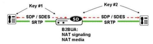
Similarly to the "Single End SRTP Termination" case above, before the request is forwarded to the callee, the SBC allocates resources and updates the SDP with proper media addresses and ports, however, at this point, the original crypto attribute is replaced with one generated by the SD.
