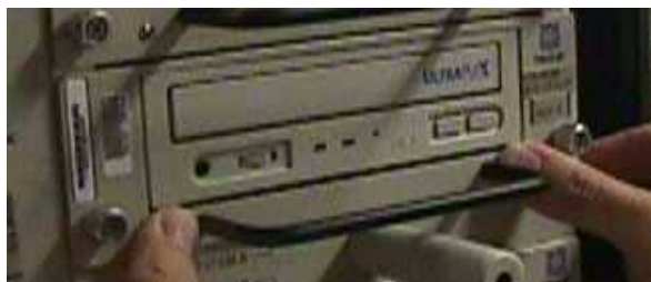
Figure 6-30. Press the Faceplate
