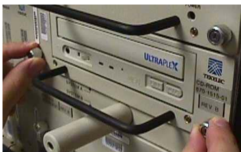
Figure 6-26. CD-ROM Drive Card Captive Screws
