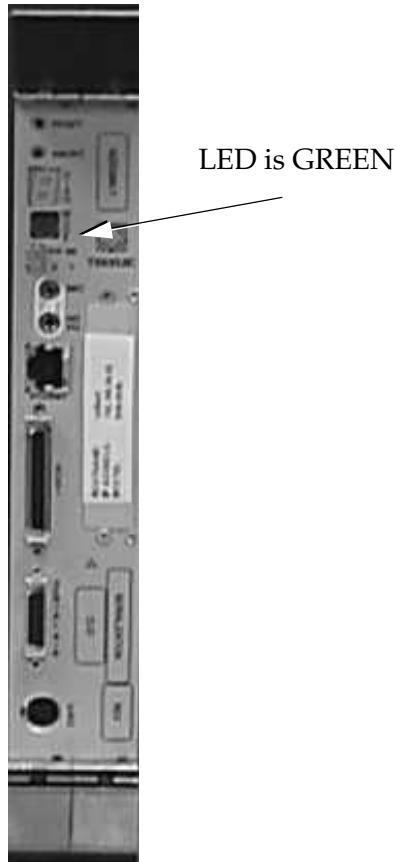
Figure 5-2. Verify LED on EOAP Is Green
