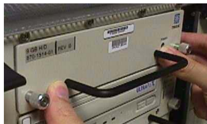
Figure 3-45. Pressing the Faceplate
