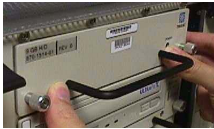
Figure 6-46. Pressing the Faceplate
