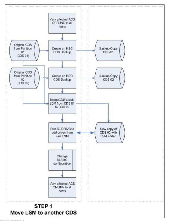
FIGURE 12-4 Process Flow to Move an Allocated LSM to Another ACS Partition
