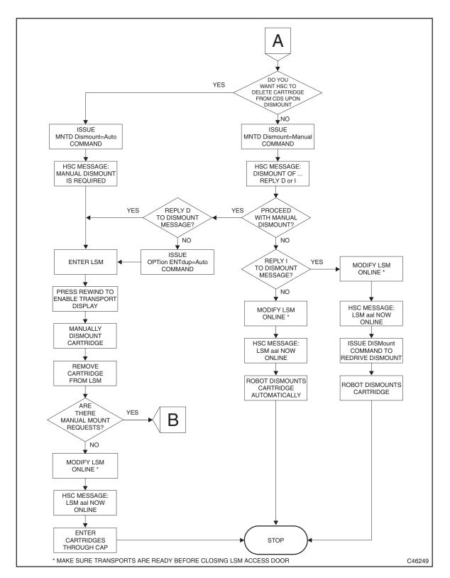
FIGURE 8-2 Manual Mode Flow Chart - Manual Dismount After Automatic Mount
