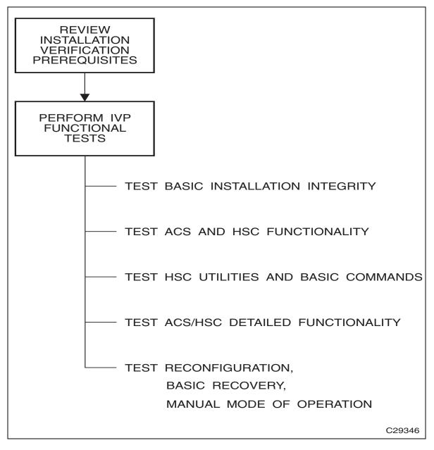
FIGURE 11-1 Installation Verification Flow Diagram
