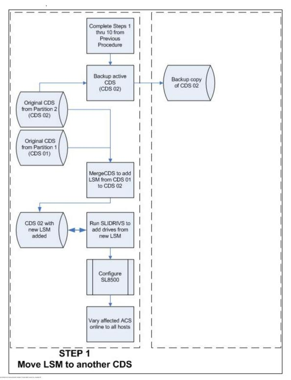
FIGURE 12-3 Process Flow to Move the Last LSM to Another ACS Partition
