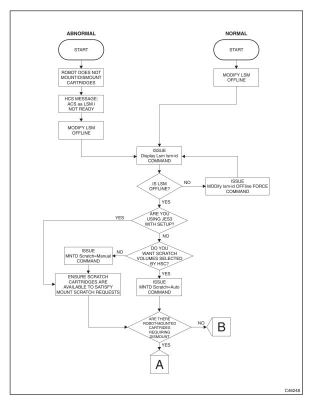
FIGURE 8-1 Manual Mode Flow Chart - Entering Manual Mode
