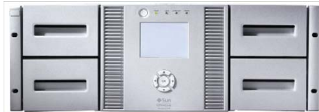
Native capacity of 72 TB with a StorageTek LTO5 tape drives
