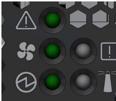
System Status LEDs* 5 Minutes After Power On
