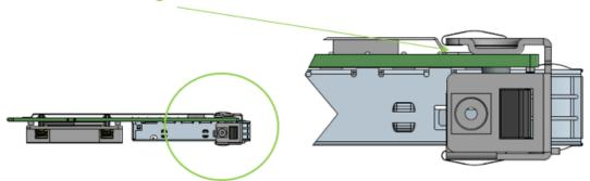
Screw on the OCP 3.0 bracket with the supplied screws that came with the new bracket kit. Use the specified torx tool type and apply the specified torque on the screws per bracket form factor.
