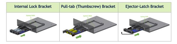
4. Push the card until connectors are in a full mate.
