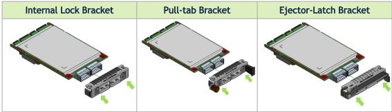
$\ensuremath{ \bigoplus}$  Do not force the bracket onto the adapter card.
