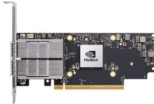
Figure 10. NVIDIA ConnectX-7 HCA
