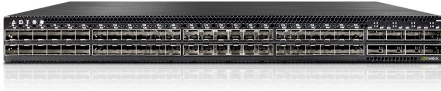
Figure 16. NVIDIA SN2201 switch
