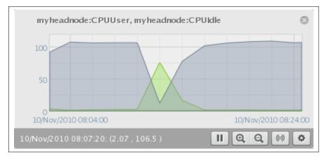
Figure 10.9: Graph Display Pane: Multiple Graphs On One Pane
