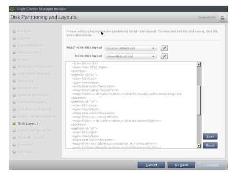
Figure 2.19: Edit Head Node Disk Partitioning
