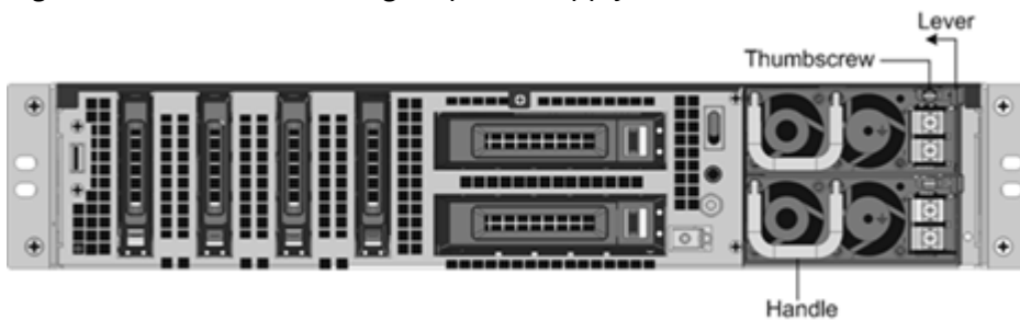
Figure 2. Remove the existing DC power supply
