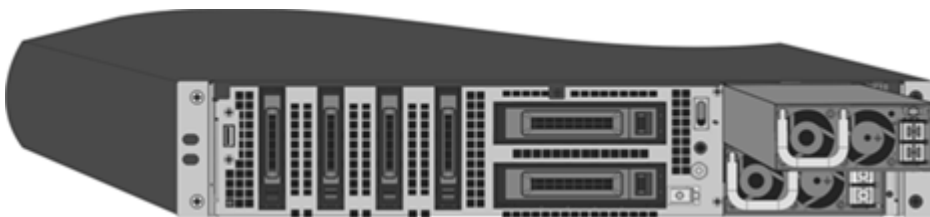
Figure 3. Inserting the Replacement DC Power Supply
