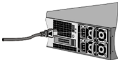
Figure 10. Insert a power cable
