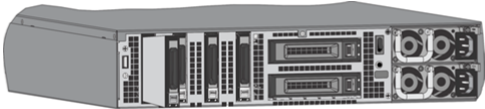
Figure 5. Insert the replacement solid-state drive
